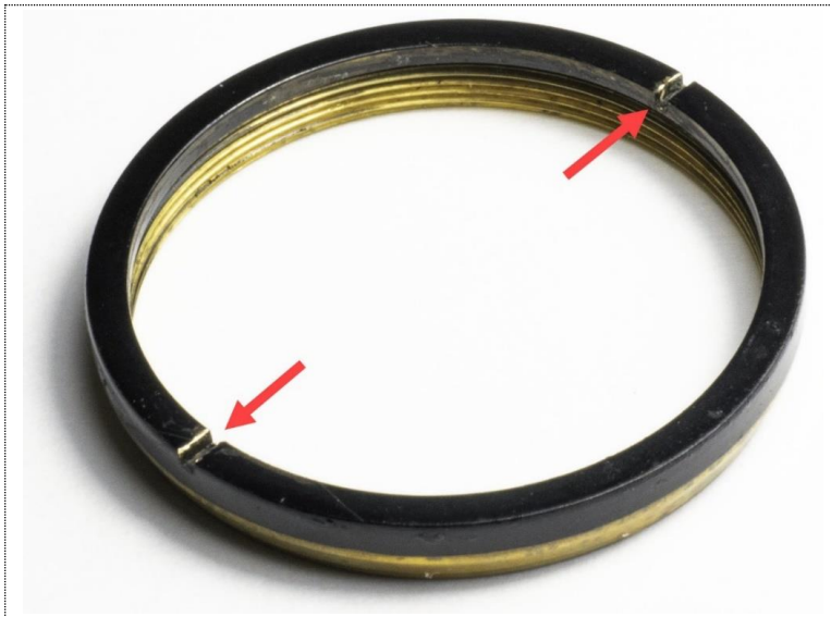
Figure 7: Closeup view of the front of the locking ring. The red arrows point to the two narrow slots into which the lens spanner tips must fit.
