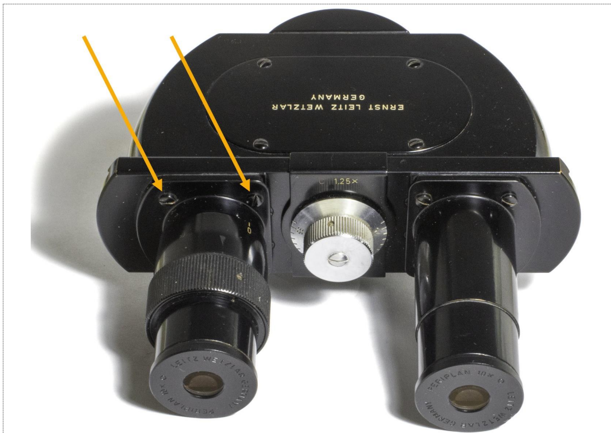
Figure 5: One of several similar binocular microscope head models from Leitz’ “black era”.
