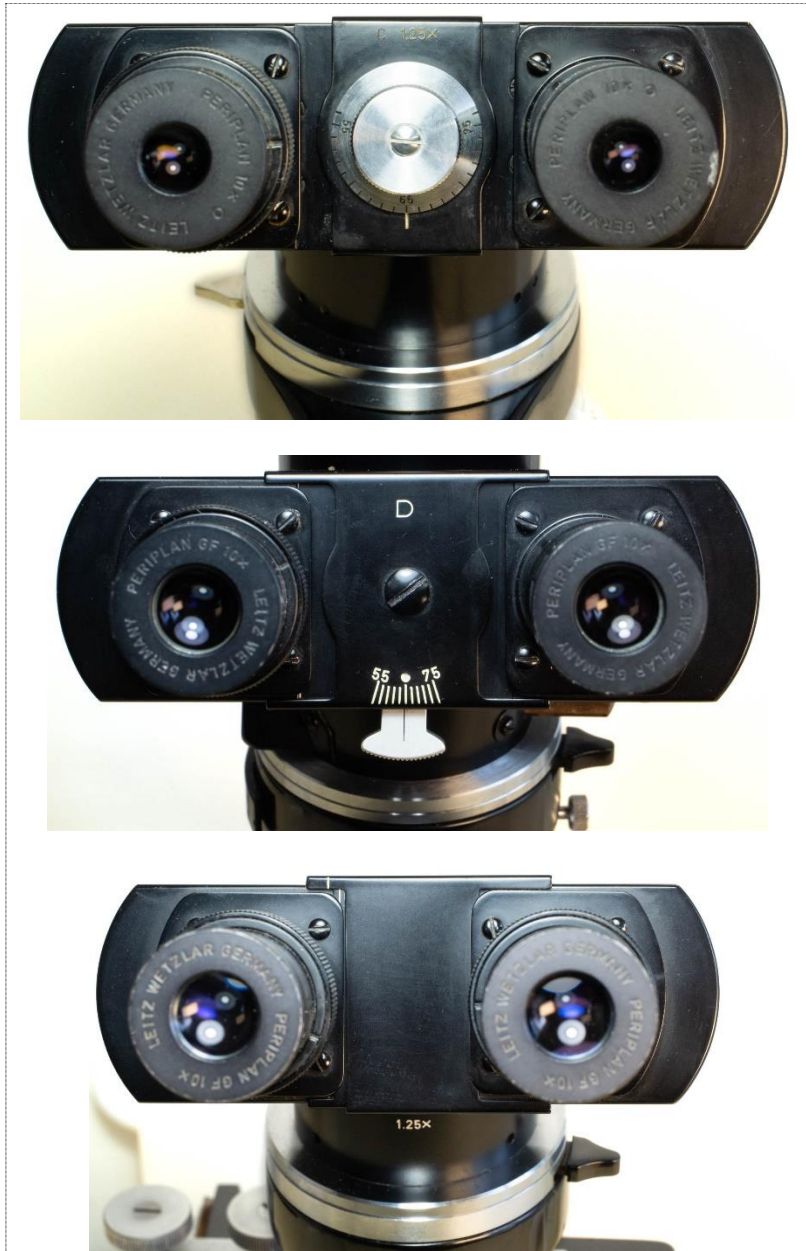
Figure 1: Three Leitz binocular/trinocular microscope heads from the “black era” with different interpupillary distance adjustment mechanisms. Top head: Interpupillary distance adjustment by a graduated knob. Middle head: Interpupillary distance adjustment by a lever with a scale. Bottom head: Interpupillary distance adjustment by manually pulling apart the eyepiece tubes against a scale (the scale is not visible in this image.)
