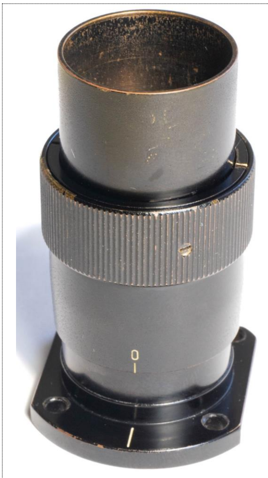
Figure 2: Focusable eyepiece tube for a head with only a diopter adjustment. The scale is a simple zero-point index that indicates where the focusable eyepiece tube has the same length as the other eyepiece tube with the fixed length.
