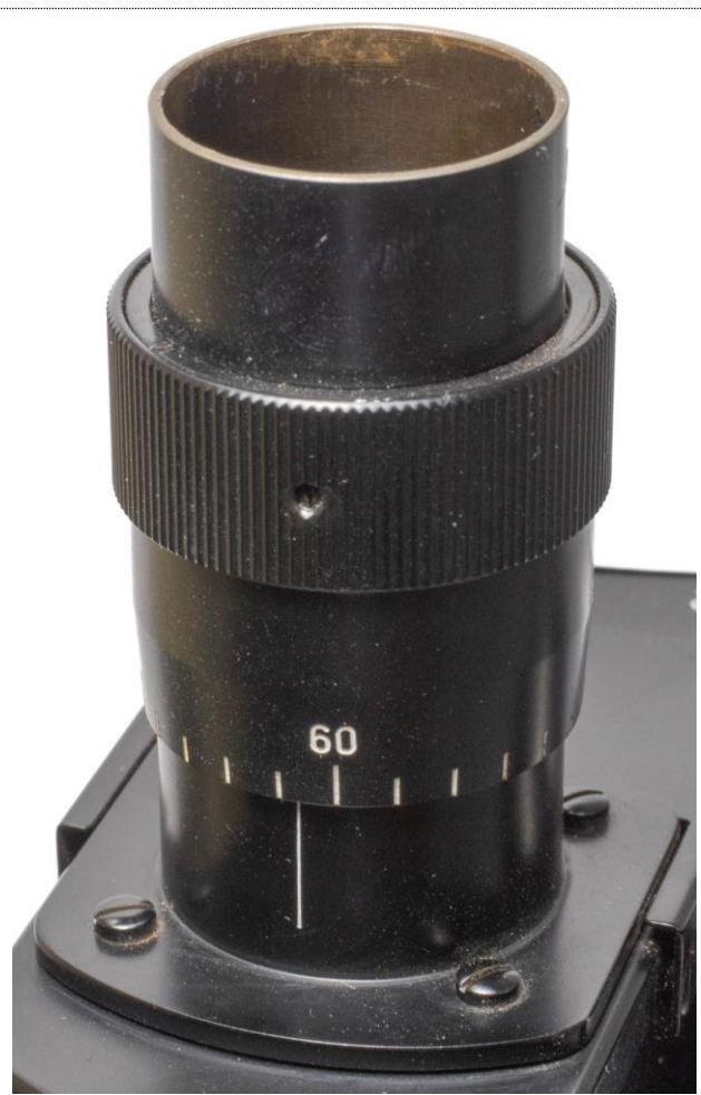
Figure 3: Focusable eyepiece tube for a head with combined diopter and interpupillary distance adjustments. The scale is numerical in units of mm interpupillary distance. After the head has been adjusted for the user's interpupillary distance, the reading from its scale is transferred to both eyepiece tube scales by turning the tubes as required. The image shows an eyepiece tube adapted to an interpupillary distance of 59½ mm.
