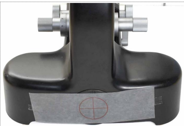
Figure 19: The lamphouse port symmetrically covered with the collimation target wax paper printout.
