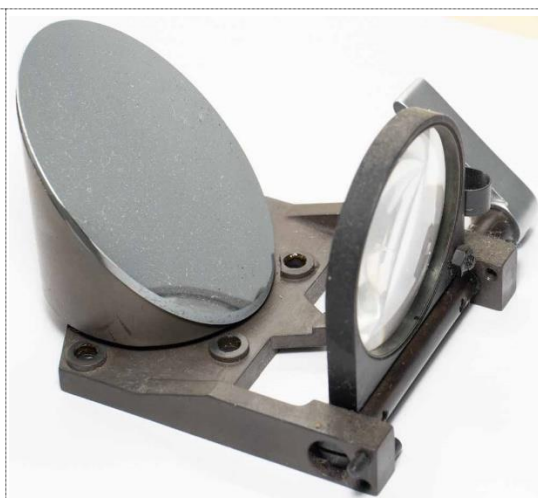
Figure 8: The removed mirror and swing-out lens holder. Here the lens is in its swing-in position.
