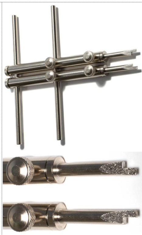
Figure 14: Camera lens spanner. Below is a closeup of the flat screwdriver type tips.
