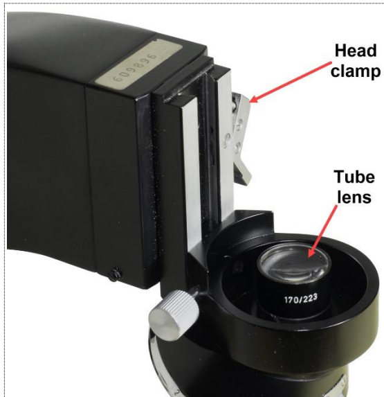
Figure 20: Ortholux nosepiece with its tube lens.
