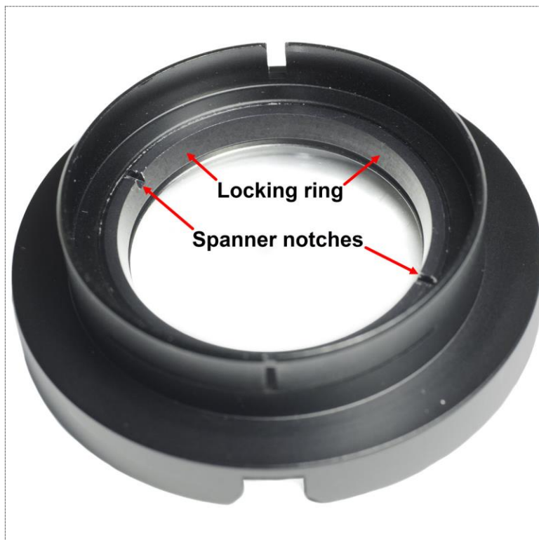
Figure 13: A filter holder where the dust protecting glass is attached by a threaded locking ring. (View from the holder's underside.)
