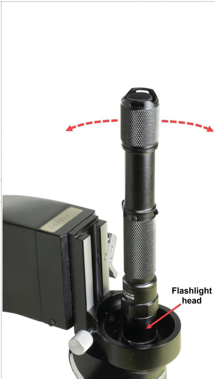
Figure 22: Ortholux nosepiece with attached flashlight.
