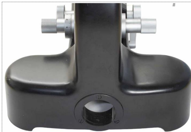
Figure 18: The empty lamphouse port on the backside of an Ortholux microscope.
