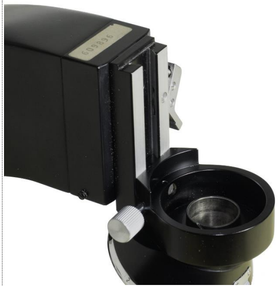
Figure 21: Ortholux nosepiece with removed tube lens.
