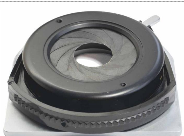
Figure 5: The removed field diaphragm unit. This diaphragm is in its middle position – the knurled thumbwheel doesn't reach outside of the width of the base plate.
