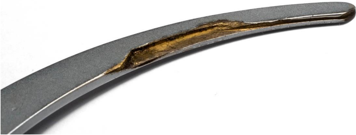
Figure 8: The underside of another even more worn object glass clamp.
