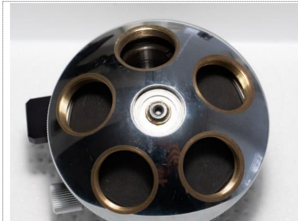
Figure 3: Nosepiece with turret; after the inner ball bearing has been removed.
