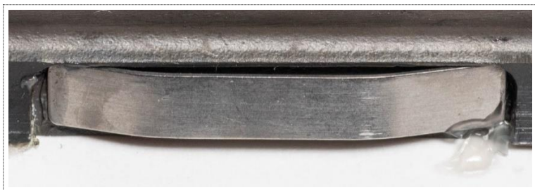
Figure 26: Closeup of one of the leaf springs in the head front's lower slide.
