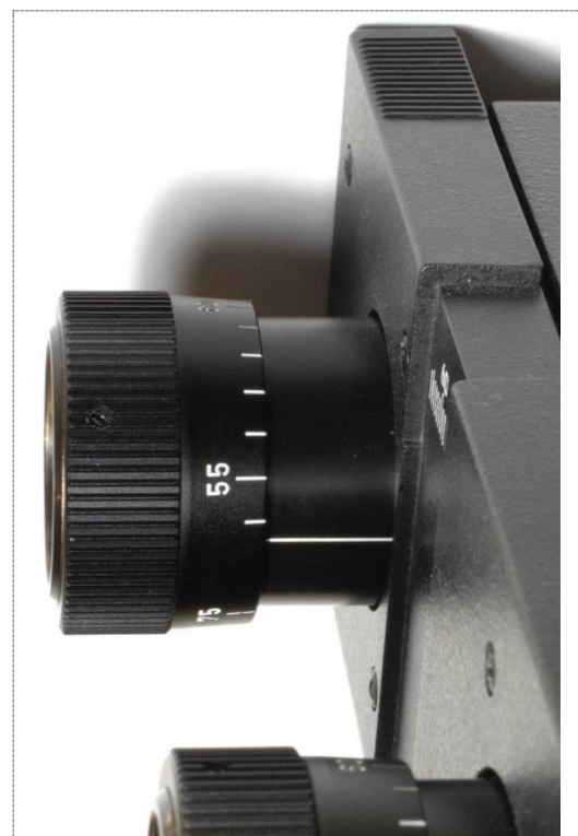
Figure 5: The left eyepiece tube with its diopter adjustment scale at the minimal interpupillary distance of 53½ mm.
