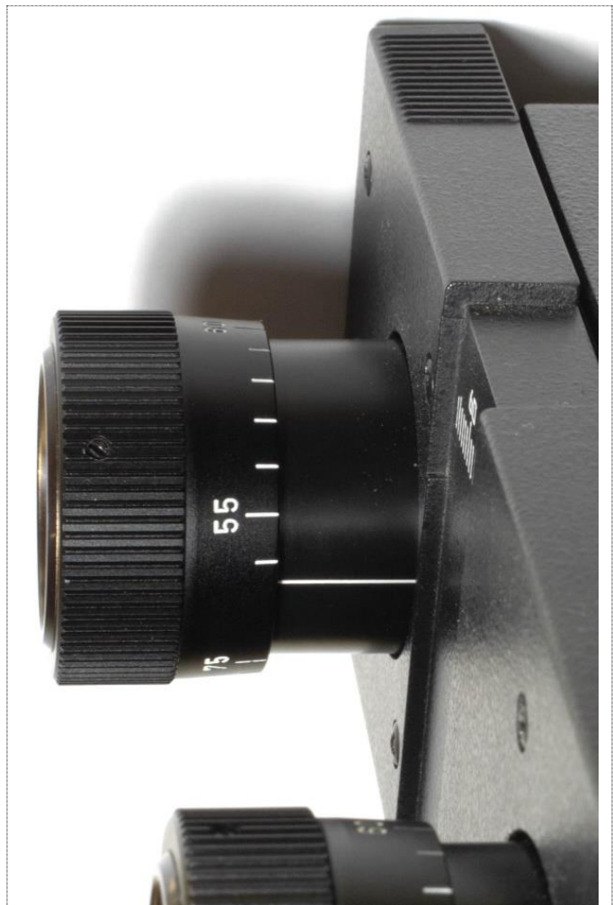
Figure 13: The left eyepiece tube with its diopter adjustment scale at the minimal interpupillary distance of 53\frac{1}{2} mm.
