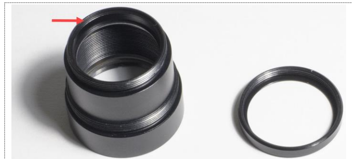
Figure 7: The graticule holder and the graticule holder ring from the field lens assembly. The red arrow points to the circular ledge where the graticule is positioned.
