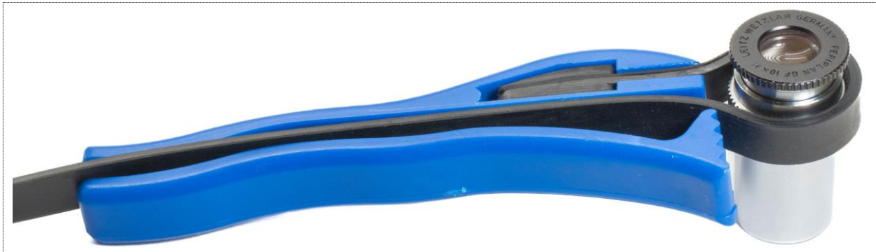
Figure 5: A small strap wrench with the strap tightly wrapped around an eyepiece.
