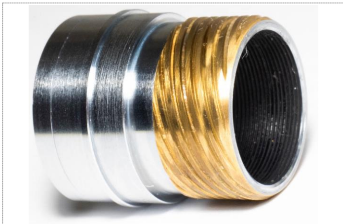
Figure 12: The eyelens focusing tube showing the helicoid thread and the inside with its black paint.
