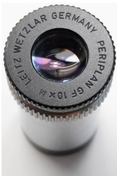
Figure 1: The Leitz Periplan GF 10x M eyepiece. View from the top.
