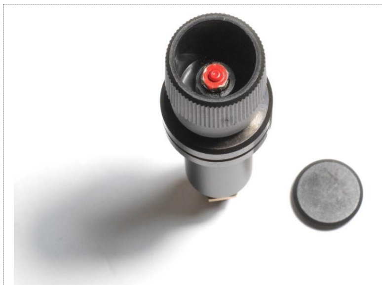
Figure 9: The x-axis knob with the cap removed. The nut is covered with a red threadlocker.
