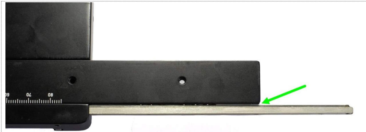
Figure 15: The x-axis slide and the bearing guide rail partly pulled out to provide a gap (green arrow) for pulling out the bearing retainer and the bearing balls.
