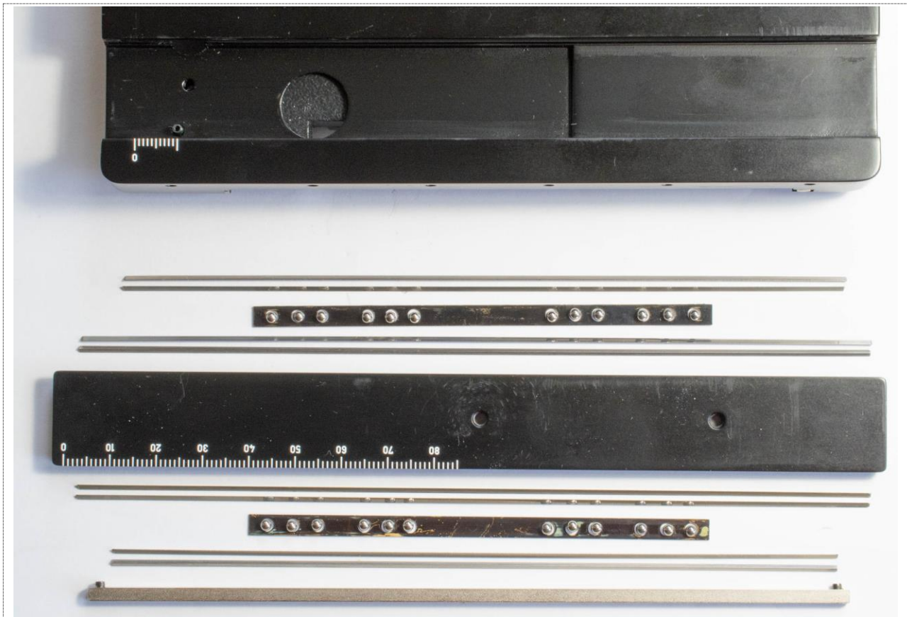
Figure 16: The x-axis slide entirely disassembled. The image shows the following, from the top and down:
