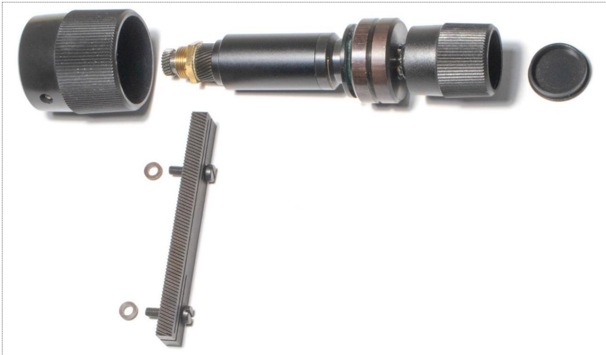
Figure 8: The coaxial stage control after removal from the stage. The previously loosened y-axis knob is to the left and the cap from the x-axis knob is to the right. Below is the y-axis rack including its screws and washers.
