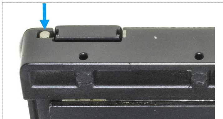
Figure 14: The side of the x-axis slide. The arrow points to the end of the ball bearing guide rail. Also refer to Figure 17.
