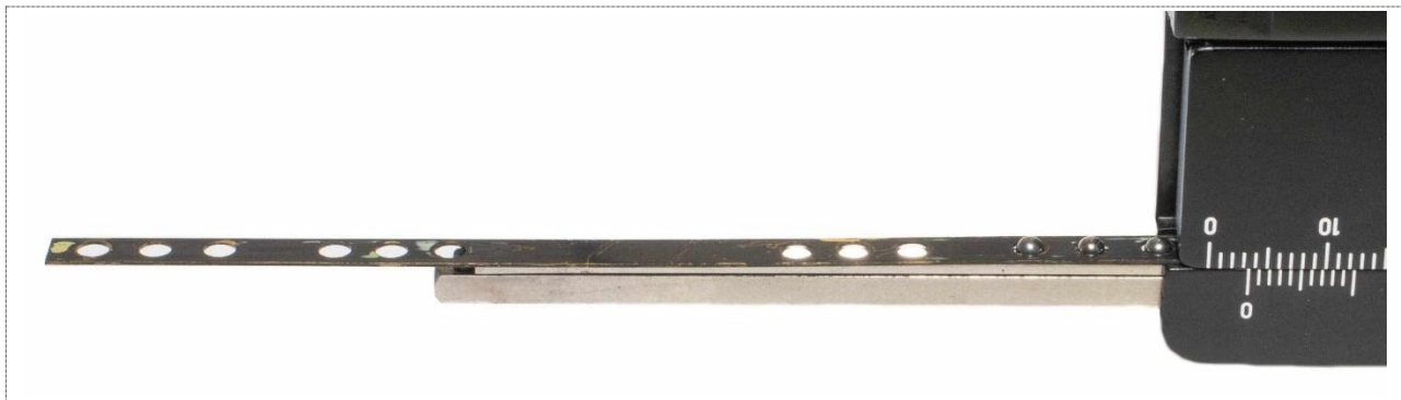
Figure 19: The guide rail pulled halfway out of the x-axis slide. Then the retainer can be inserted on top of it, and the bearing balls can be added.
