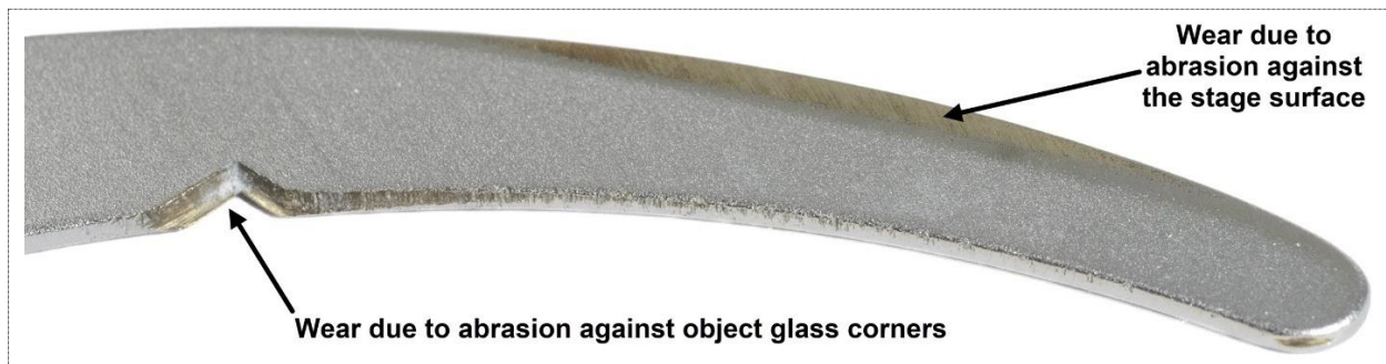
Figure 24: Closeup of the underside of a well used object glass clamp.
