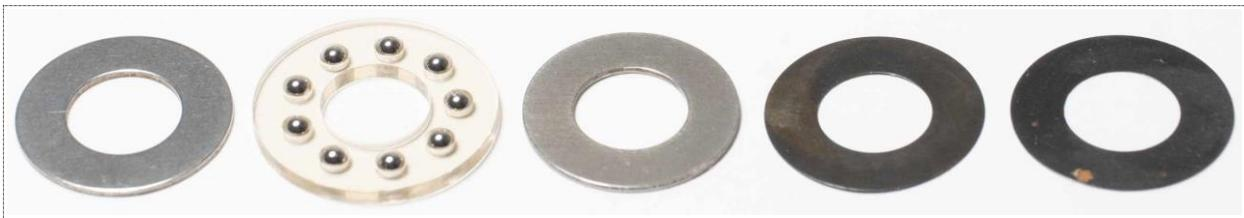
Figure 14: The components of the ball bearing that carries the turret. Starting from the bottom of the turret axle, and from the right side of the image:
