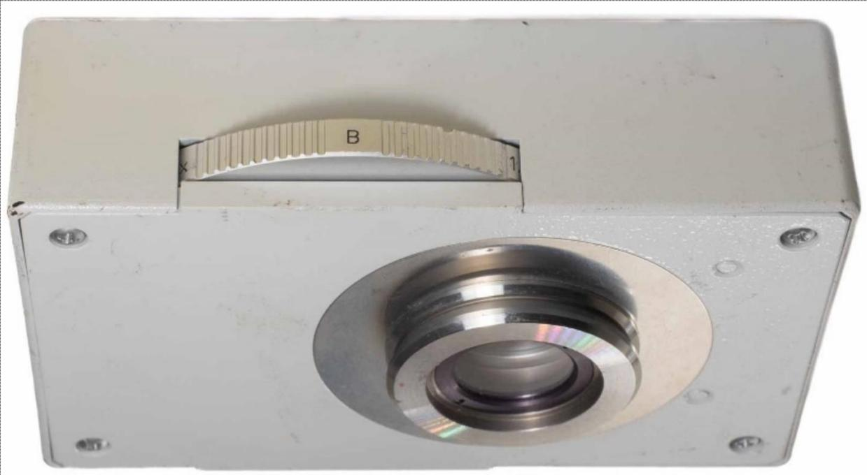
Figure 2: View of the Magnification Changer's bottom side with its 42 mm male dovetail mount.
