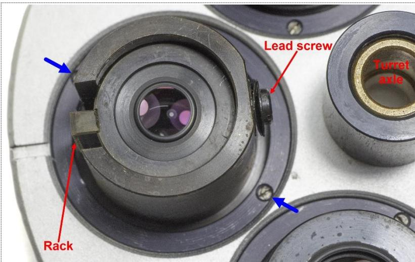
Figure 10: The Bertrand lens case on the turret.
