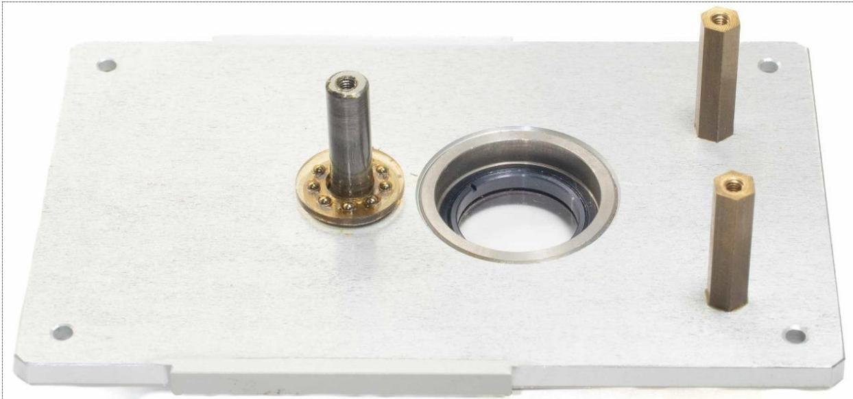
Figure 13: The bottom plate after the turret has been removed. Parts of the turret axle's ball bearing are now visible.
