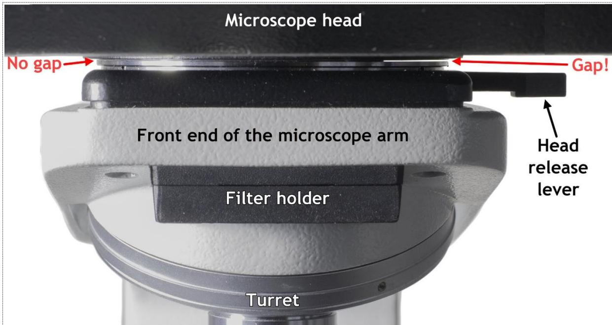
*Figure 16: A small gap between the underside of the head and the collar of the head mount reveals that the head is not properly attached. The head in this image is slightly tilted.*
