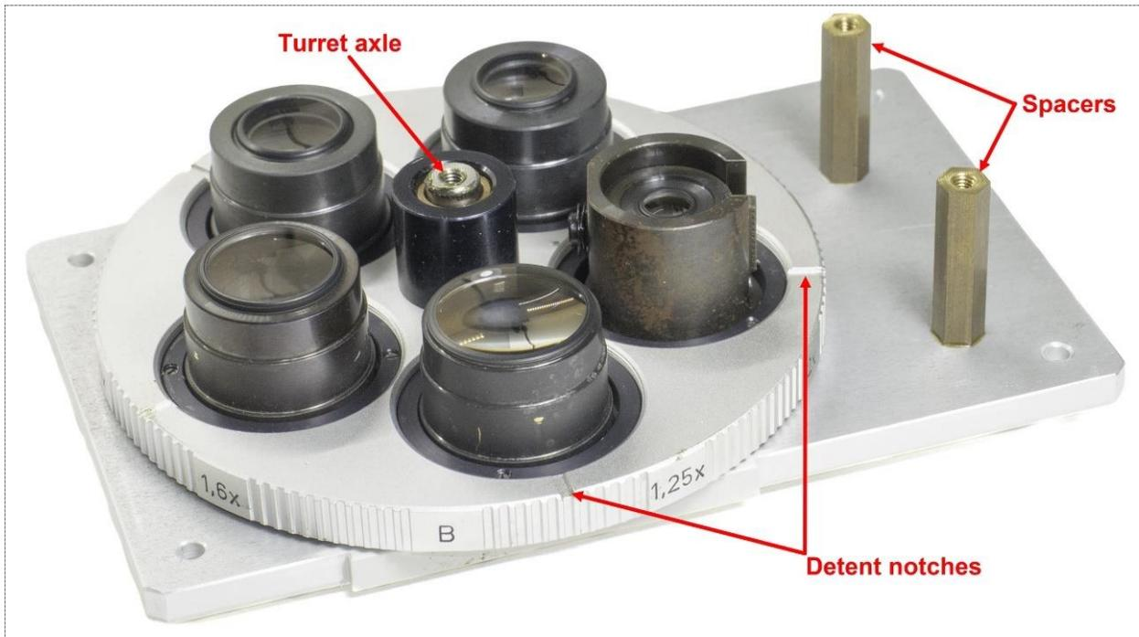
Figure 11: View of the turret sitting on the bottom plate's turret axle.
