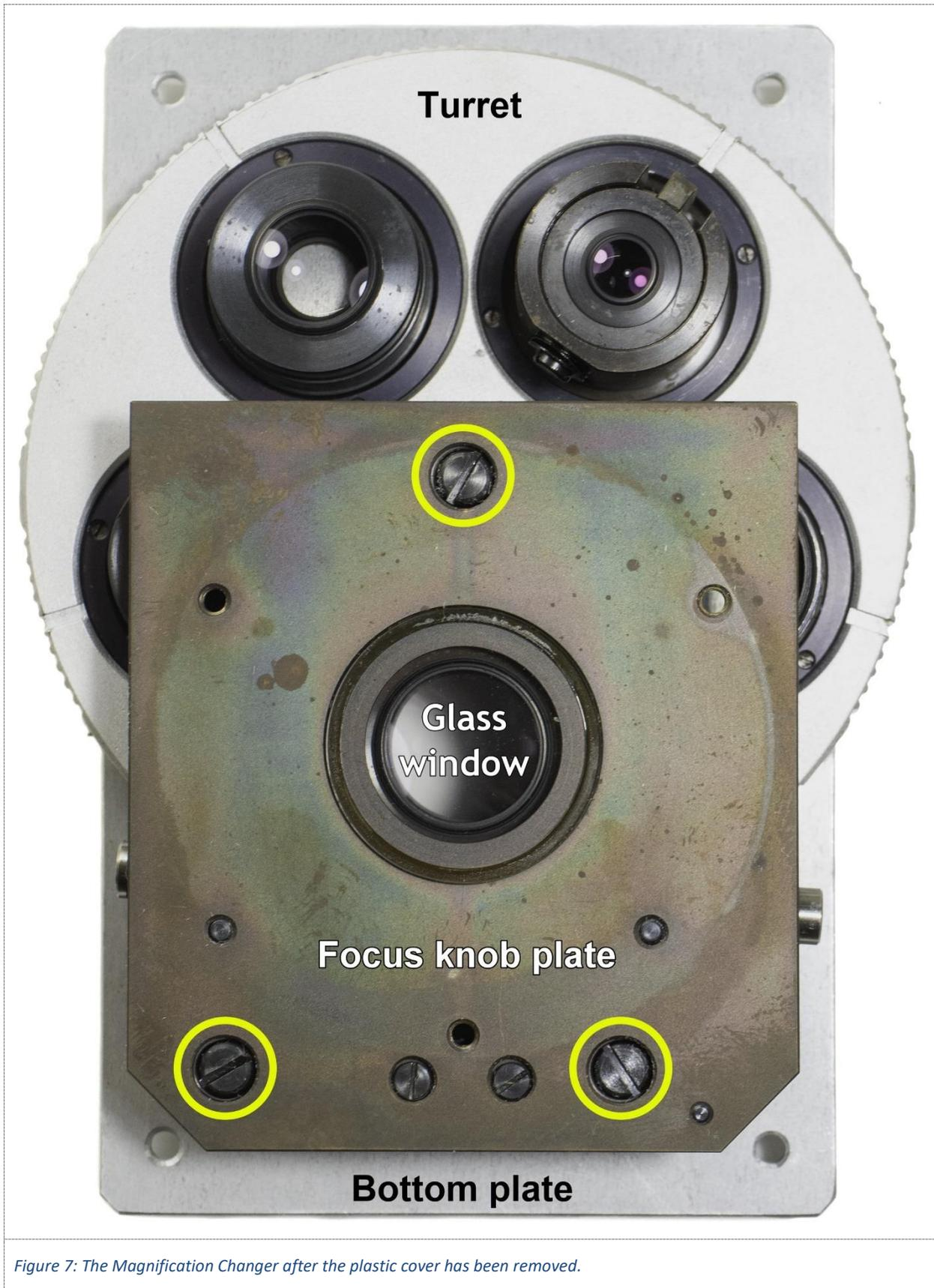
Figure 7: The Magnification Changer after the plastic cover has been removed.
