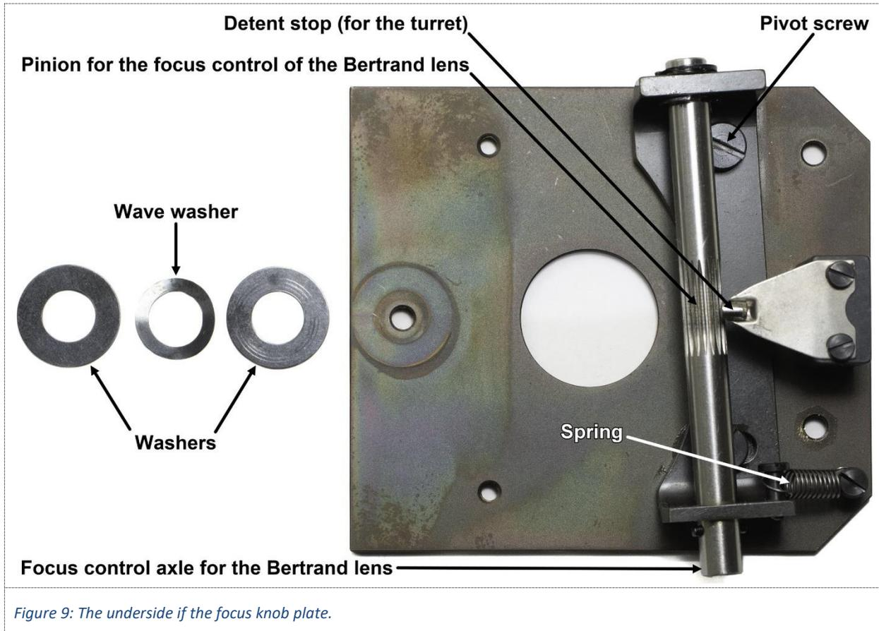
*Figure 9: The underside of the focus knob plate.*
