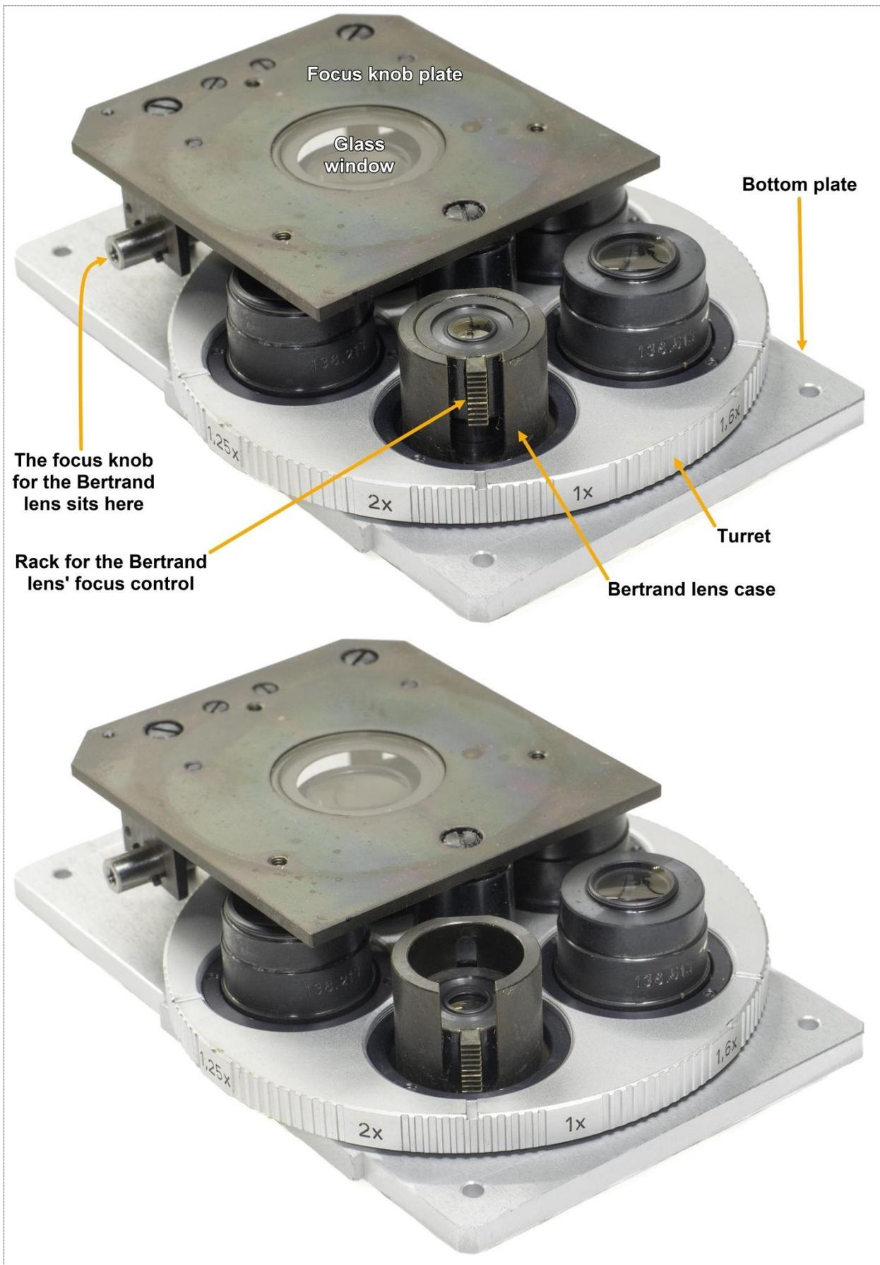
Figure 8: Oblique view of the Magnification Changer after the plastic cover has been removed. The only difference between the two images is that the Bertrand lens case is shown with different focus settings.
