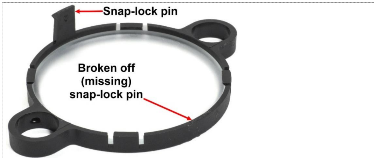
Figure 6: The push-on diffuser disc (frosted glass filter) with its black plastic frame. It is attached to the light port of Lamphouse LH 20.
