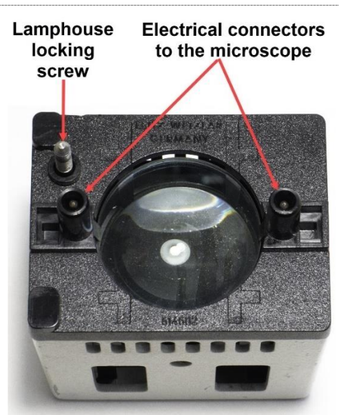
Figure 4: The light port on the front of the lamphouse. Note the connection plugs with the integrated electrical connectors.
