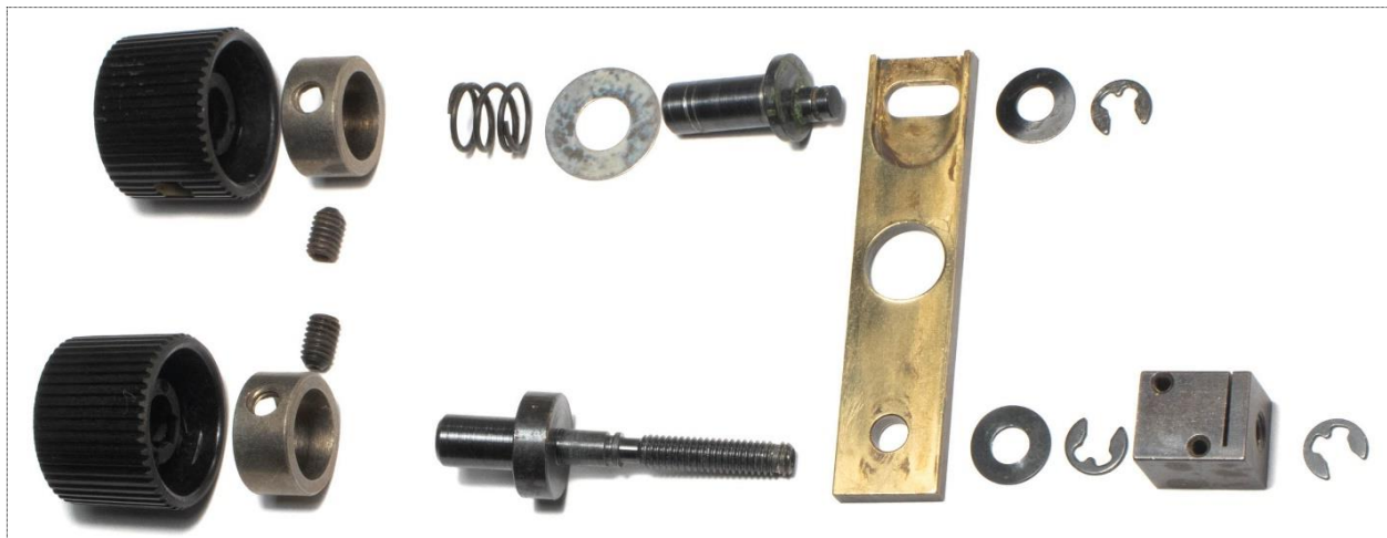
Figure 8: Exploded view of the lamp adjustment mechanism. The vertical adjustment parts on the top of the image, and the lateral adjustment parts on the bottom of the image. The vertical slide is the shared part.
