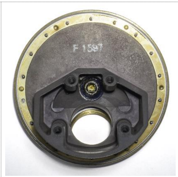
Figure 11: The turret, after the threaded turret locking ring and the bearing race have been removed. The bearing retainer and the bearing balls are now visible.
