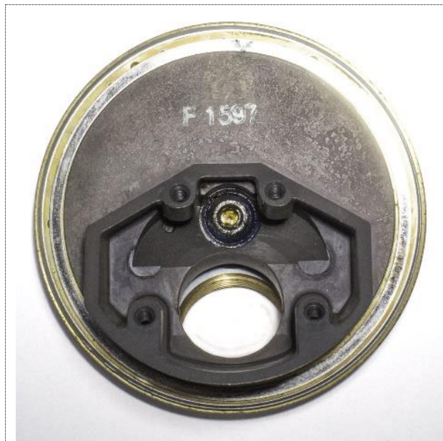
Figure 10: The turret, after the threaded turret locking ring has been removed. The large turret ball bearing is now visible. The bearing balls are not visible because they are below the ball bearing race.
