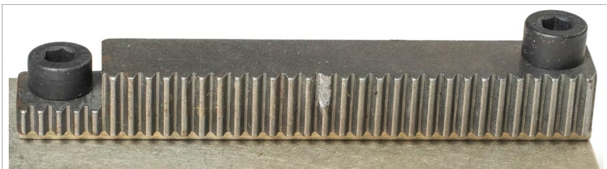
Figure 11: A focus rack with shipping damage.
