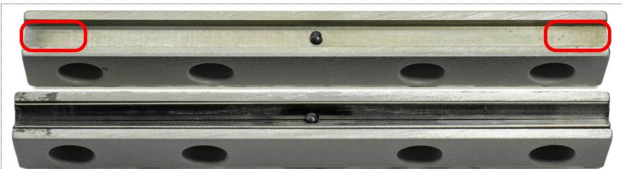
Figure 32: The upper bearing guide shows where in the groove the "glue" grease should be applied. The lower bearing guide shows the guide after the bearing race rails have been attached.
