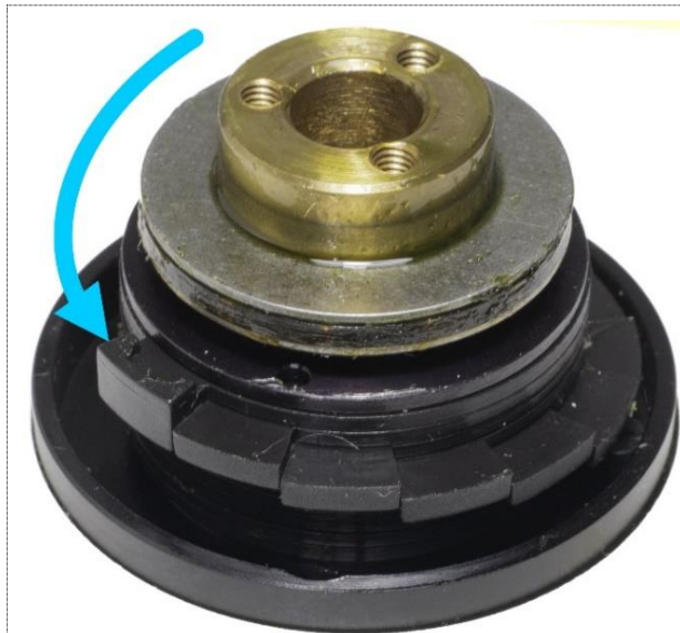
Figure 28: The arrow shows where one of the screws inside of the left coarse focus knob catches the top ring protrusion. (Note: This image shows the base of a Dialux 20 microscope, but the general idea also applies for Laborlux D.)
