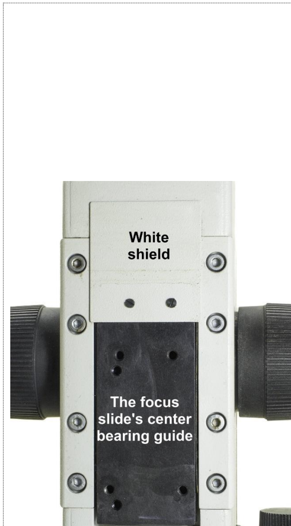
Figure 7: The microscope's focus slide after the stage holder has been removed.
