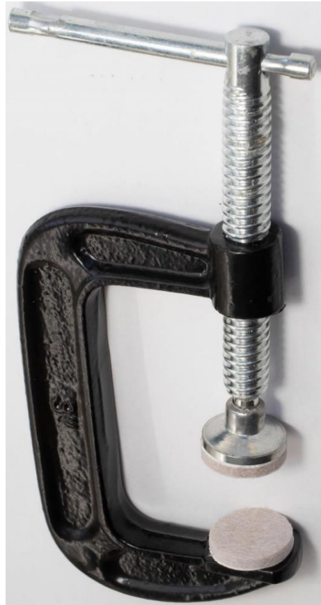
Figure 35: A C-clamp with self-adhesive protectors attached to the gripping edges.
