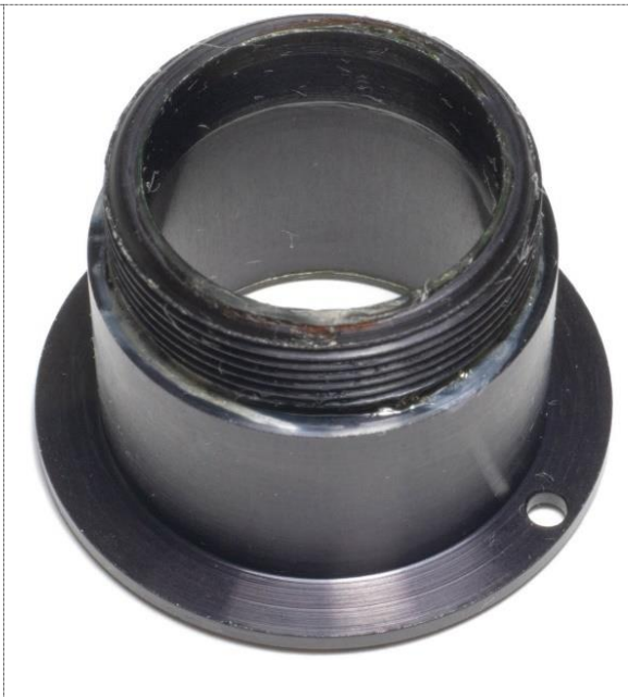
Figure 25: The black guide tube from the focus range limiting mechanism. The flange is facing downward in this image. The guide tube holds the stack of the 10 plastic rings (removed here.)
