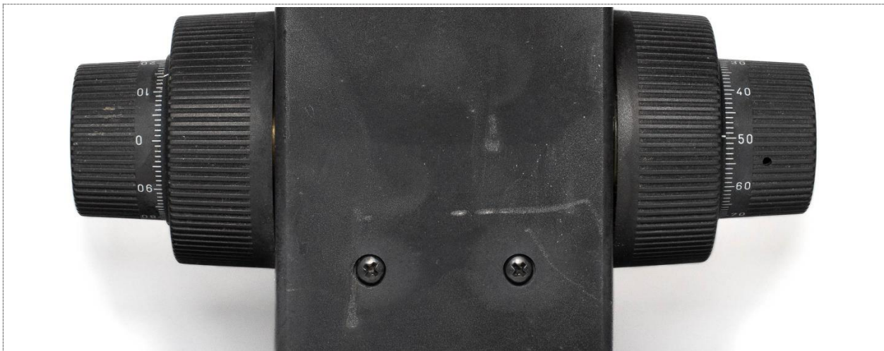
Figure 2: Laborlux S coaxial focus controls viewed from the backside of the microscope.
