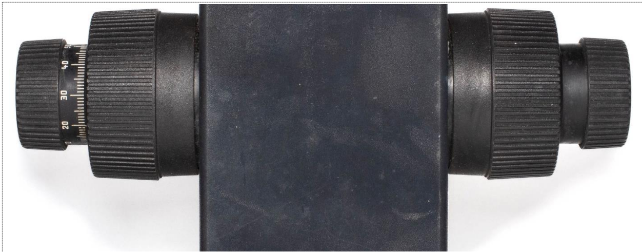
Figure 1: Laborlux D coaxial focus controls viewed from the backside of the microscope.
