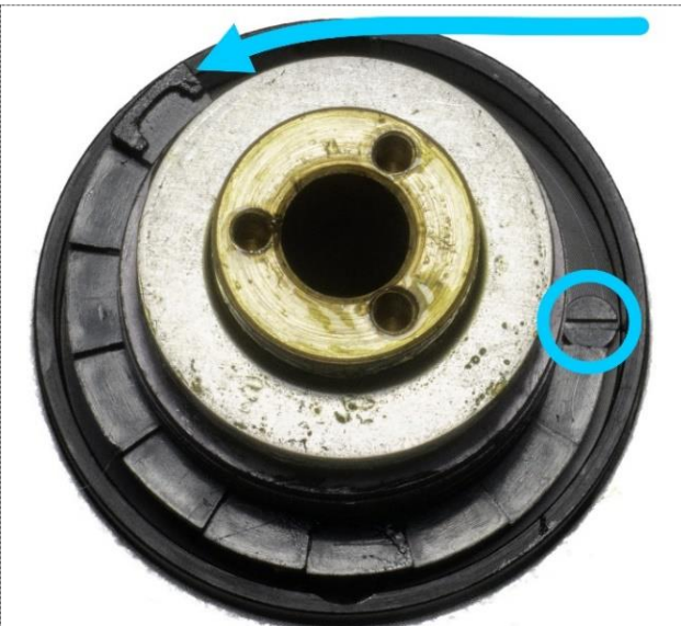
Figure 29: The entire train of the rings have here reached the focus range limit by colliding with the screw (blue circle) that sticks up from the left focus control base. (Note: This image shows the base of a Dialux 20 microscope, but the general idea also applies for Laborlux D.)
