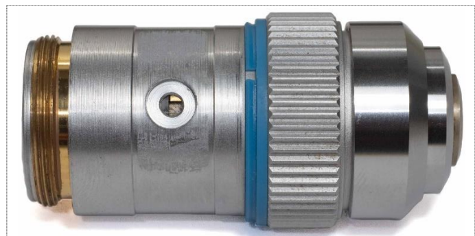
Figure 10: The lens housing groove slightly off sideways when viewed through the stop plug hole.
