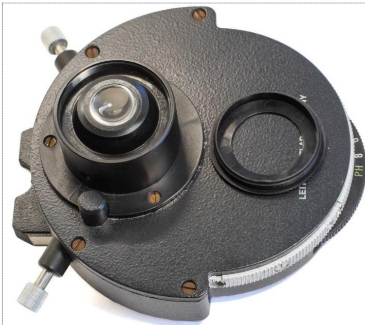
Figure 9: Condenser UKL with the protective ring removed and put to the side.
