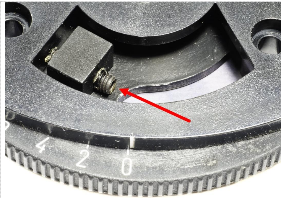
Figure 25: Close-up of the aperture diaphragm range limiting mechanism. The red arrow indicates the head of the adjustment screw.
