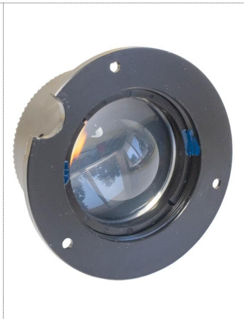
Figure 10: View from the underside of the condenser top.
