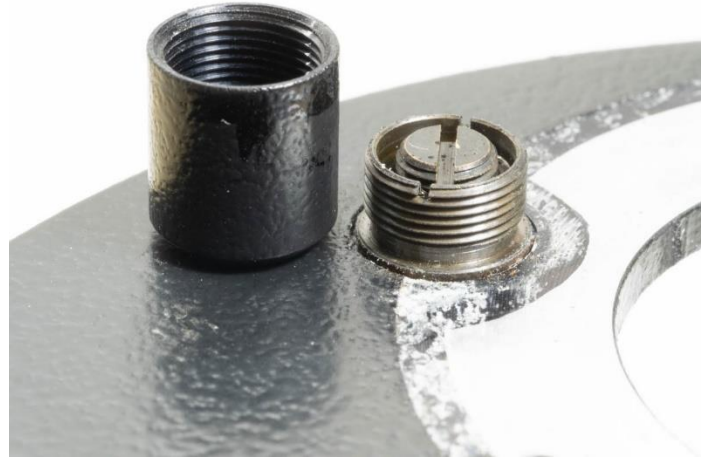
Figure 29: The detent stop adjustment screw is accessible after the cap has been removed.
