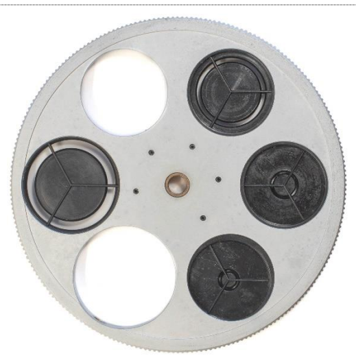
Figure 6: View of the underside of the light ring turret. This turret has one light ring for darkfield microscopy and three light rings for phase contrast microscopy.
