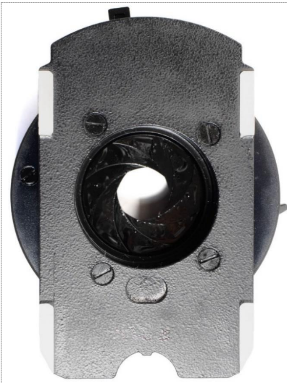
Figure 18: View of the underside of the condenser with its dovetail mount.
