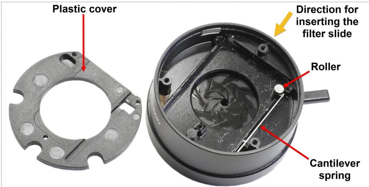
Figure 17: View down into the condenser's filter slide compartment after the plastic cover has been removed. This is where the filter slide is inserted.
