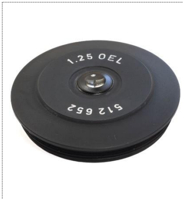
Figure 2: The n.a. 1.25 oil immersion cap for condenser no. 56.
