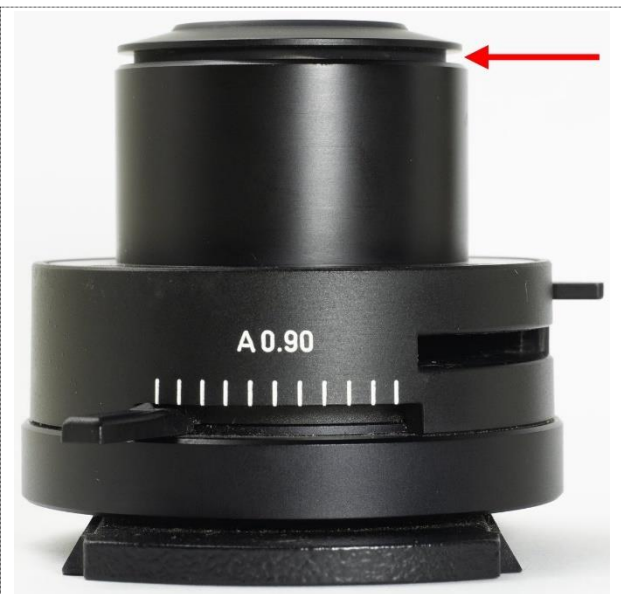
Figure 26: Condenser no. 56 with the immersion oil cap attached over the top lens as far as it goes. The red arrow points to the gap left between the condenser and the cap.
