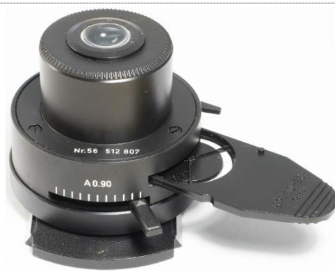
Figure 3: Condenser no. 56 with a darkground slide inserted in the position where it is outside of the optical path.
