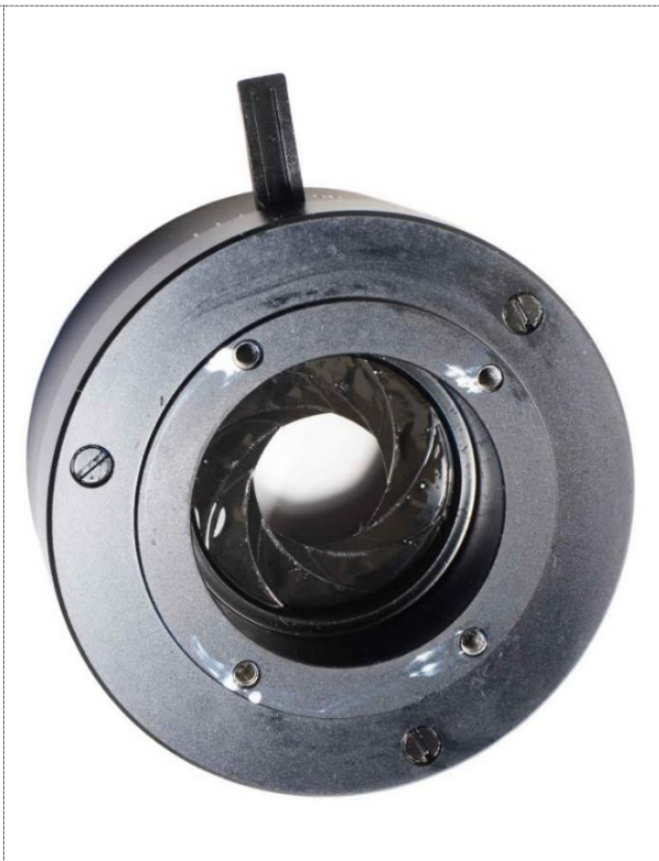
Figure 19: The underside of the condenser after the dovetail mount has been removed. This is the underside of the aperture diaphragm base.
