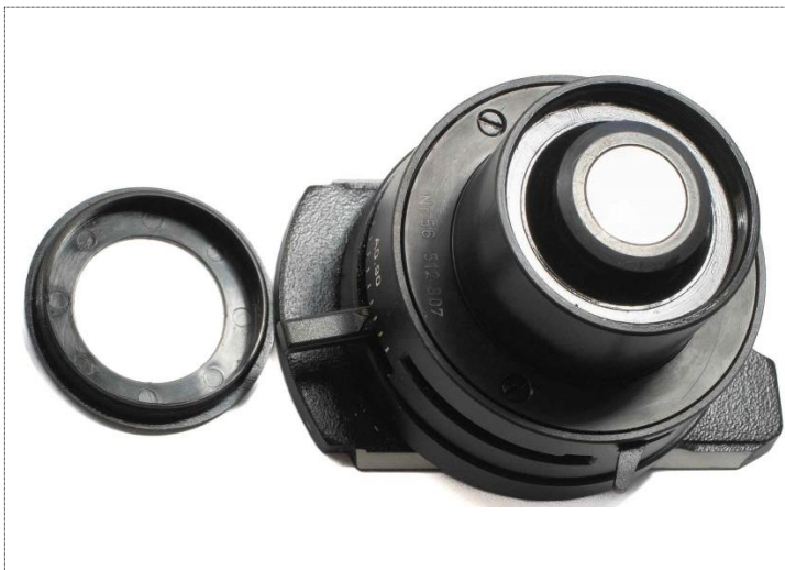
Figure 9: Condenser no. 56 with the protective ring removed.
