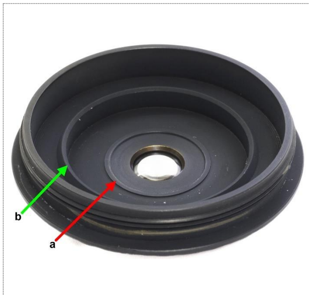
Figure 25: Oil immersion cap n.a. 1.25 viewed from the underside. When attached to the condenser the ring at "a" is touching the surface of the top lens. The ring at "b" goes outside of the top lens and doesn't touch any part of it.
