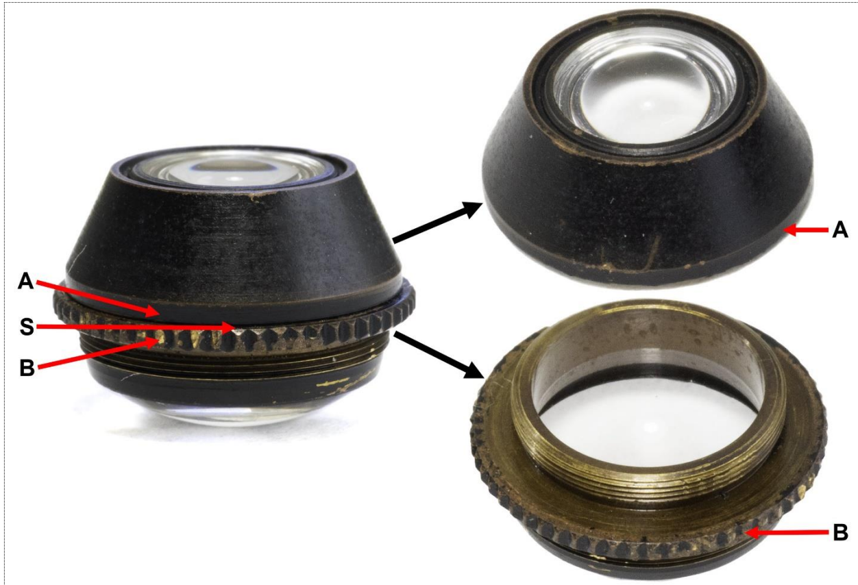
Figure 57: How the top element can be separated into two halves.
