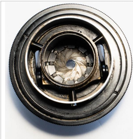
Figure 21: View on the underside of the aperture diaphragm block. The image shows the aperture diaphragm on the inside of the block.
