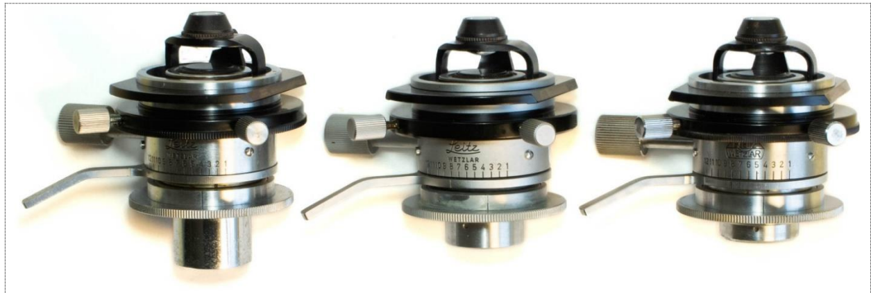
Figure 5: Three Berek condensers with slightly different lower collector lens designs.
