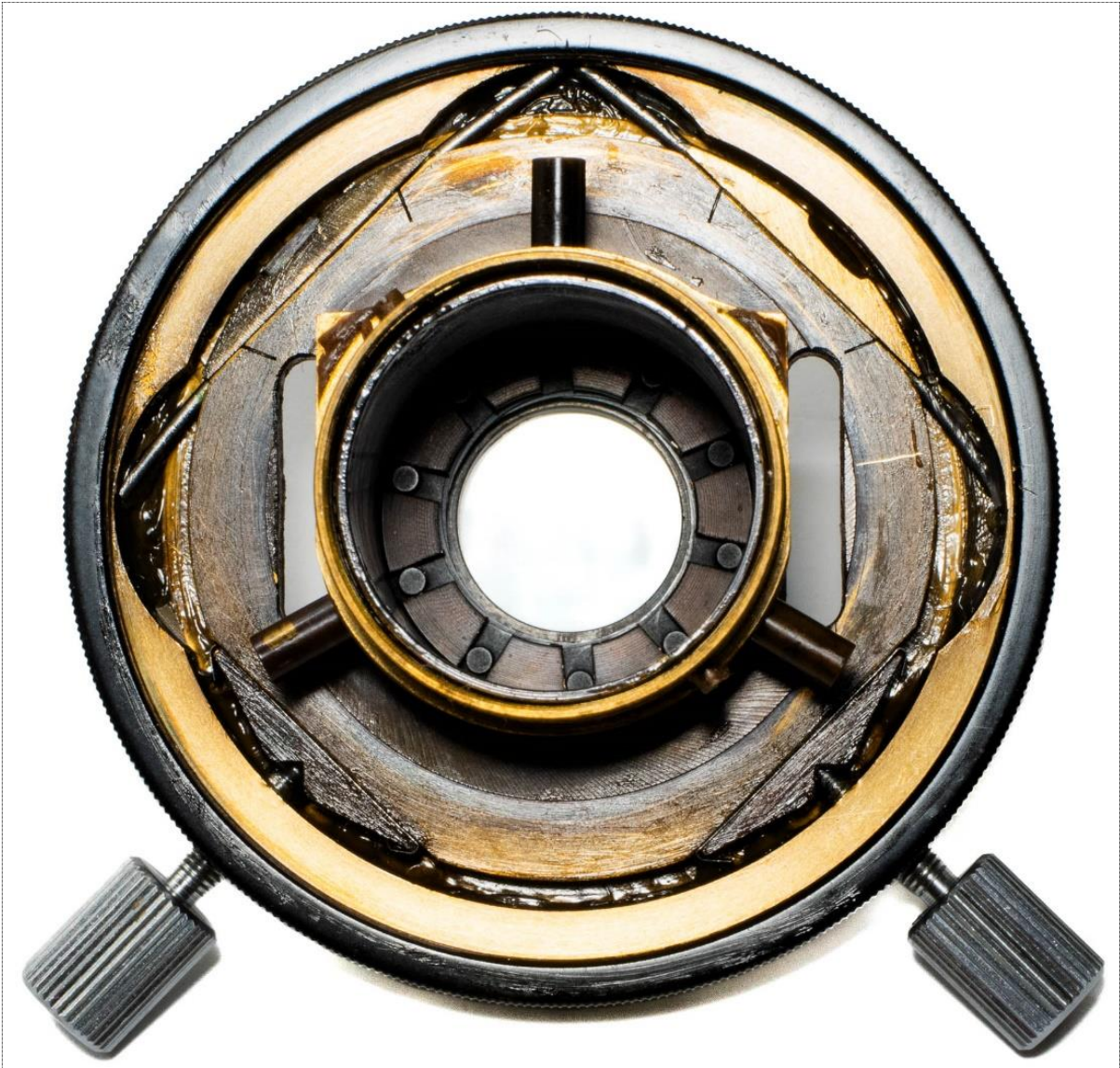
Figure 28: The centering slide in the aperture diaphragm block after the cover has been removed.
