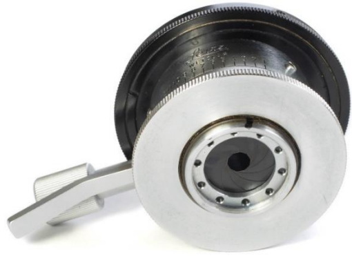
Figure 14: View from the bottom of the Berek condenser. The lower collector lens has been removed and the field diaphragm (almost closed here) is accessible.
