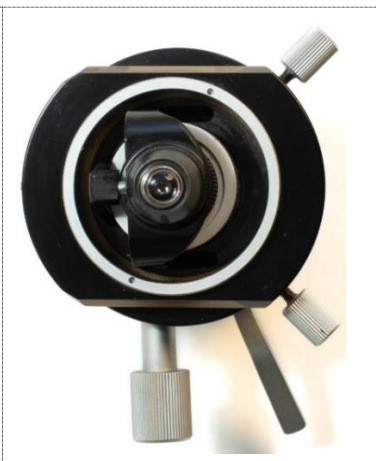
Figure 7: Berek condenser, view from the top, with the swing-out top element engaged.
