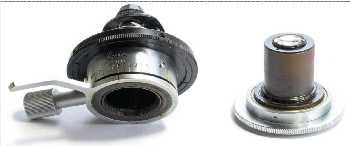
Figure 16: The Berek condenser divided into its two blocks – the aperture diaphragm block (left) and the field diaphragm block (right.)
