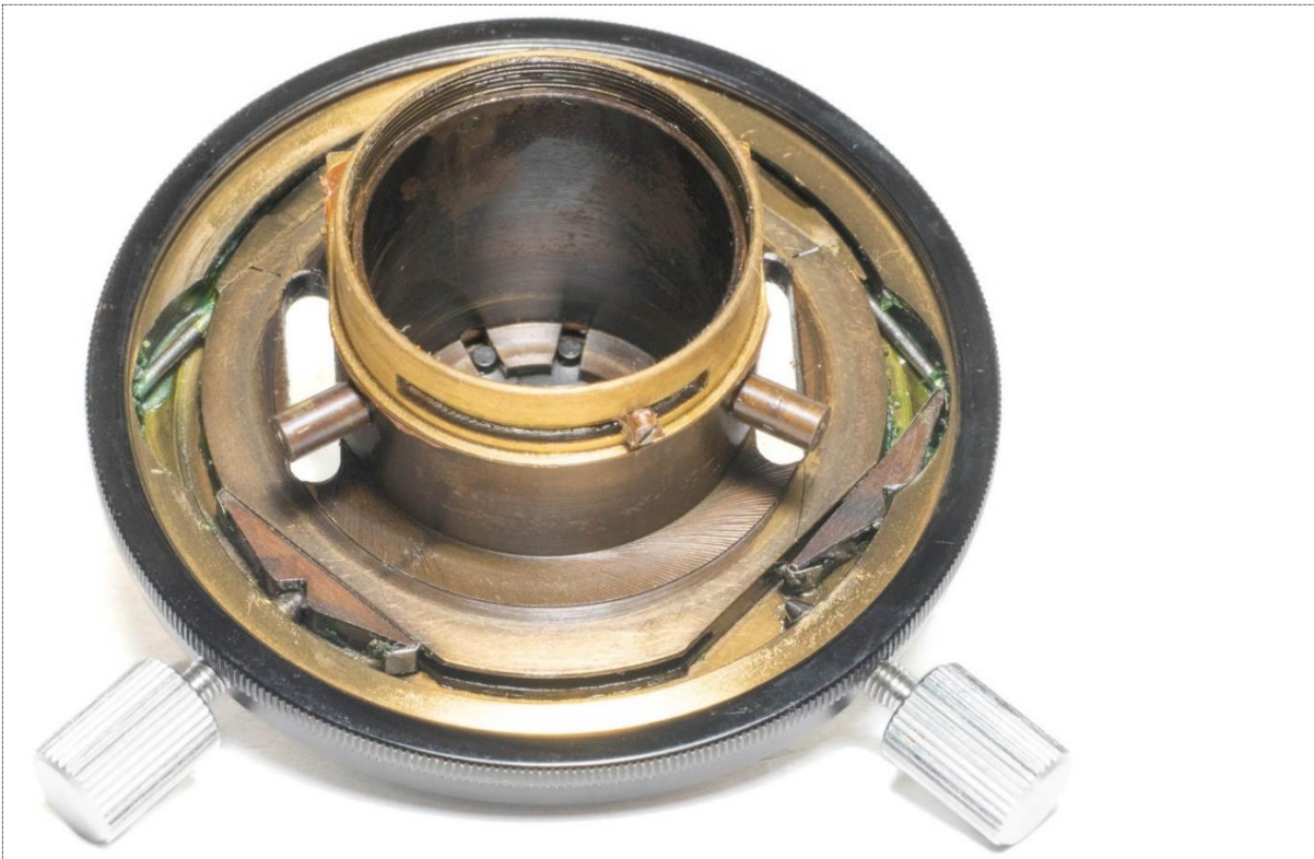
Figure 29: The centering slide demonstrating a mechanical failure. The left centering screw and pusher are intact, but the right pusher has slipped away from the left centering screw and become wedged in the slide. The slide is stuck.
