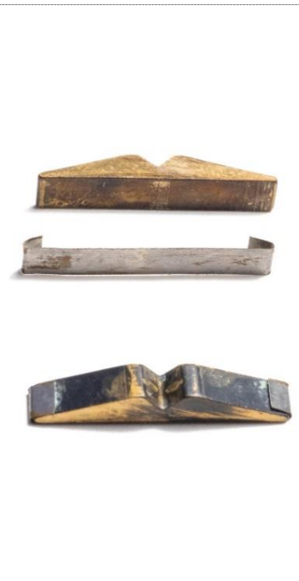
Figure 31: Close-up view of the centering mechanism's pushers and steel liners. On the top the parts are separated, on the bottom the parts are assembled.
