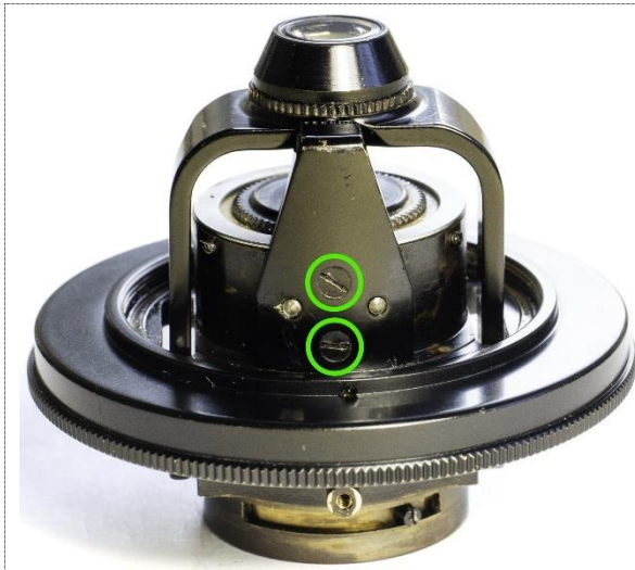
Figure 24: The two outside screws that hold the top element stop (within green circles.)
