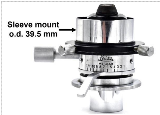
Figure 4: Berek condenser with a sleeve mount.
