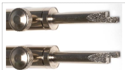
Figure 26: Flat tips on a camera lens spanner.
