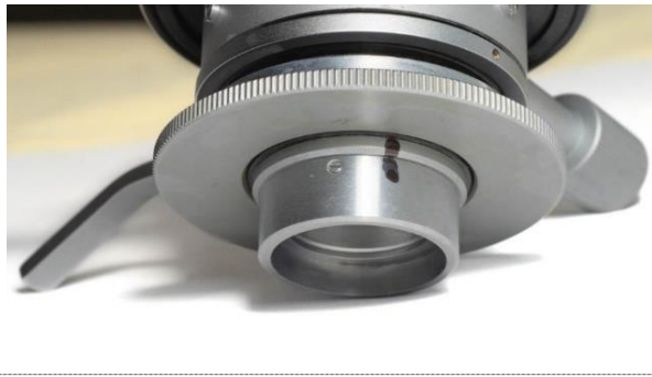
Figure 13: The lower collector lens at the bottom of the Berek condenser. One of the three small centering screws is visible.
