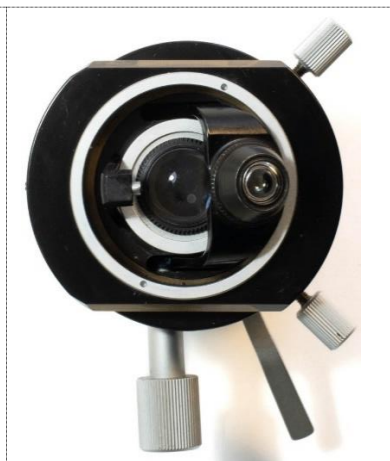
Figure 8: Berek condenser, view from the top, with the swing-out top element folded to the side.
