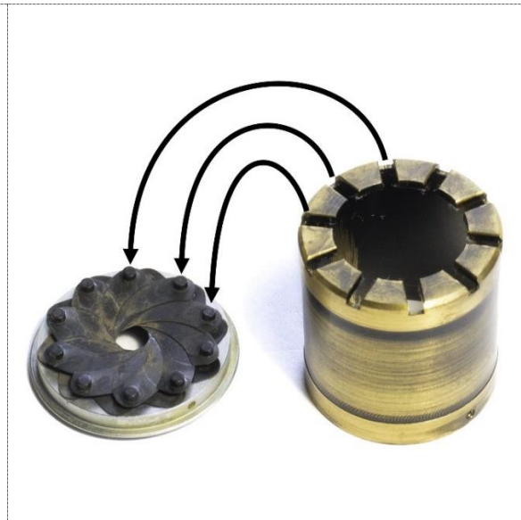
Figure 22: The aperture diaphragm blades anchored to the base plate (left side of the image) and the cylindrical aperture diaphragm actuator (right side of the image). The arrows show how the pivot pins on the blades fit into the slots at the end of the actuator.
