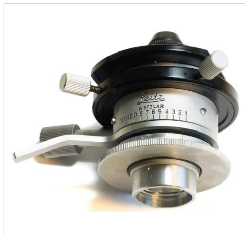
Figure 6: Berek condenser, view obliquely from below.
