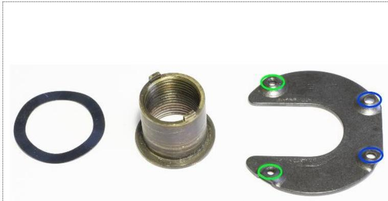
Figure 16: The wave washer, the bushing, and the “horseshoe”.
