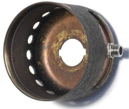
Figure 17: The lamp holder removed from the lamphouse.
