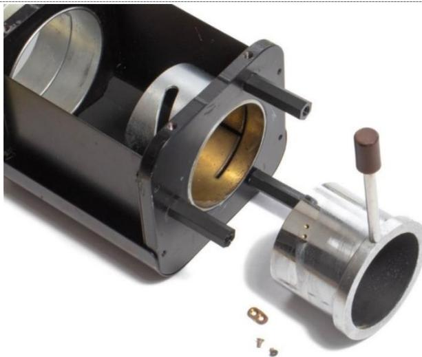
*Figure 25: The collector removed from the lamphouse. The removed helicoid guide is shown below the collector.*
