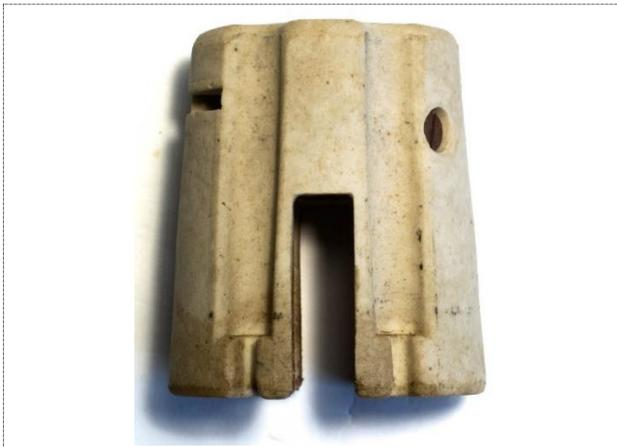
Figure 11: The lamp socket viewed from the side. The screw seen in the upper right part of the socket is a part of the electrical connection to the bulb cap.
