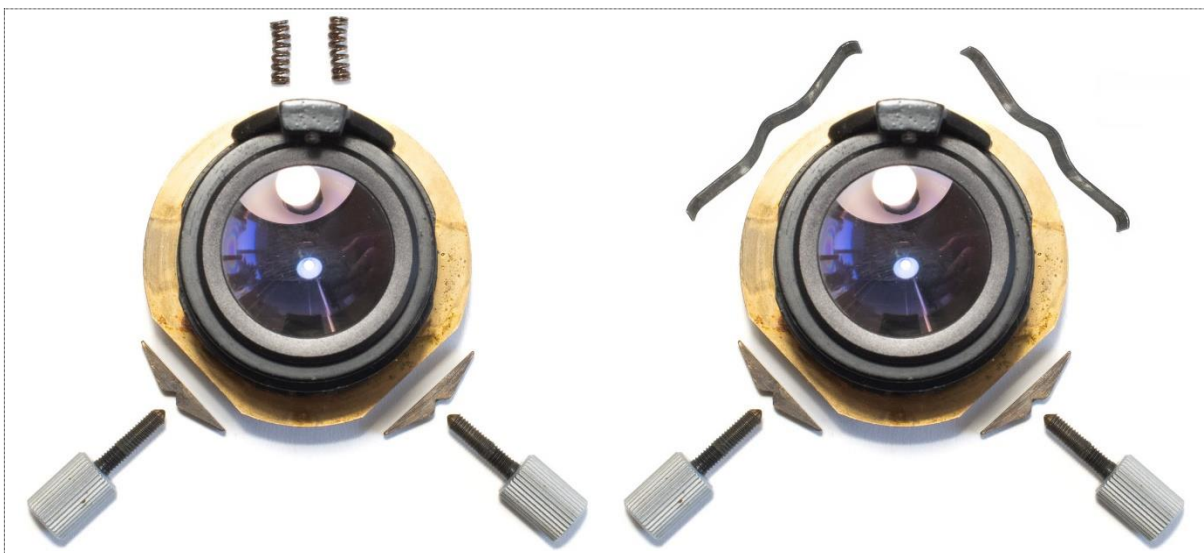
Figure 18: Exploded view (from above) of the condenser core with the parts of the centering mechanism (the compression spring variant to the left and the leaf spring variant to the right.)
