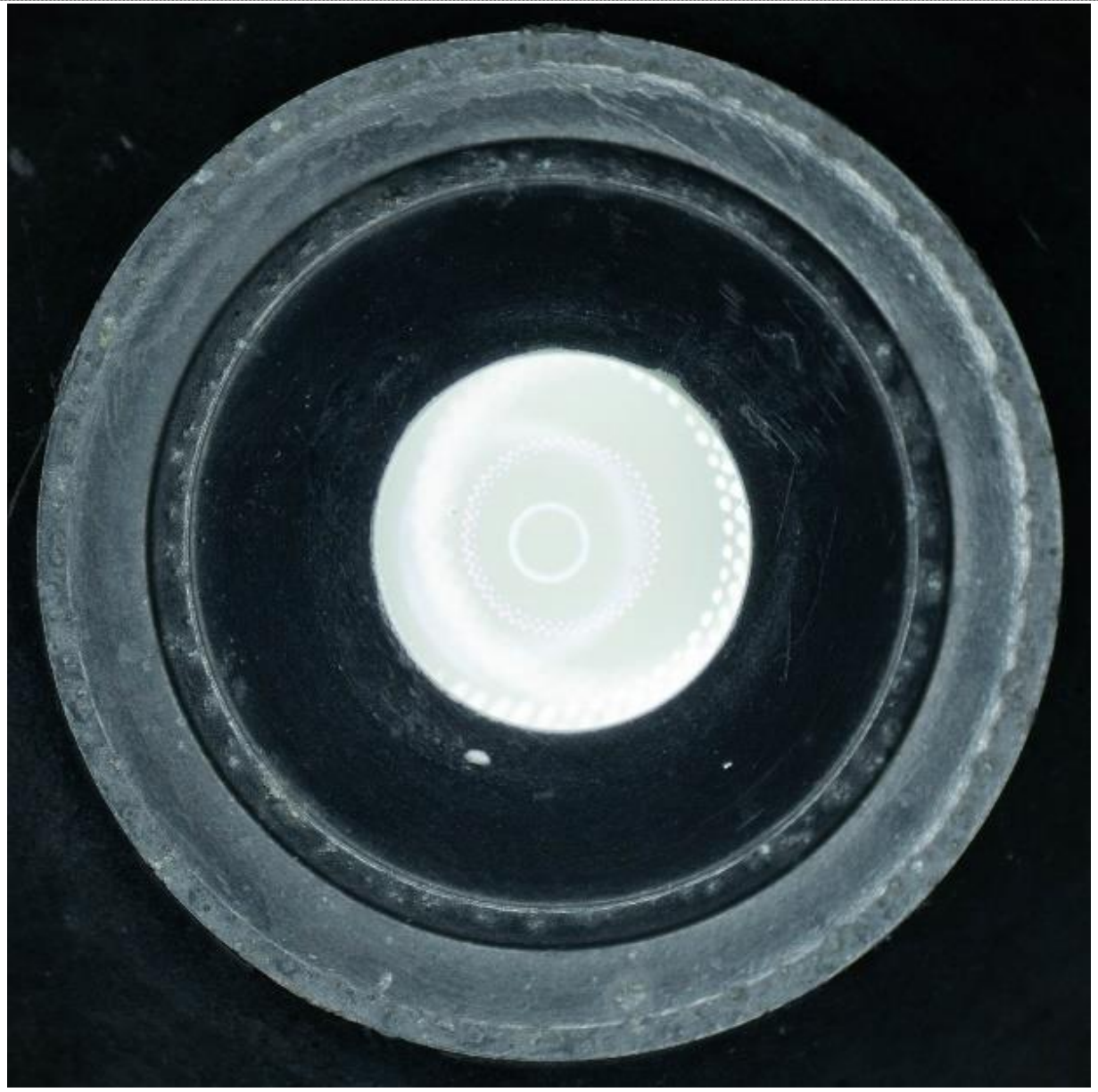
Figure 33: An “Achr 0.90” top element viewed from above in a stereo microscope. The black paint is largely intact. The bright dotted circles on the clear lens surface are reflections of the circular LED illumination.
