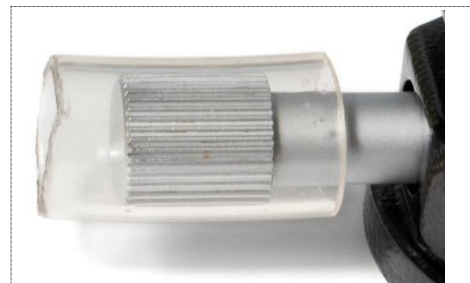
Figure 13: The swing-out knob for the top element protected with a piece of PVC tube.
