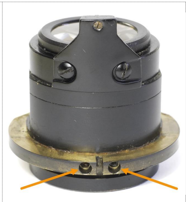
Figure 21: The removed condenser core viewed from the backside. The arrows point to the holes for the compression springs. (The top element yoke has prematurely been removed.)
