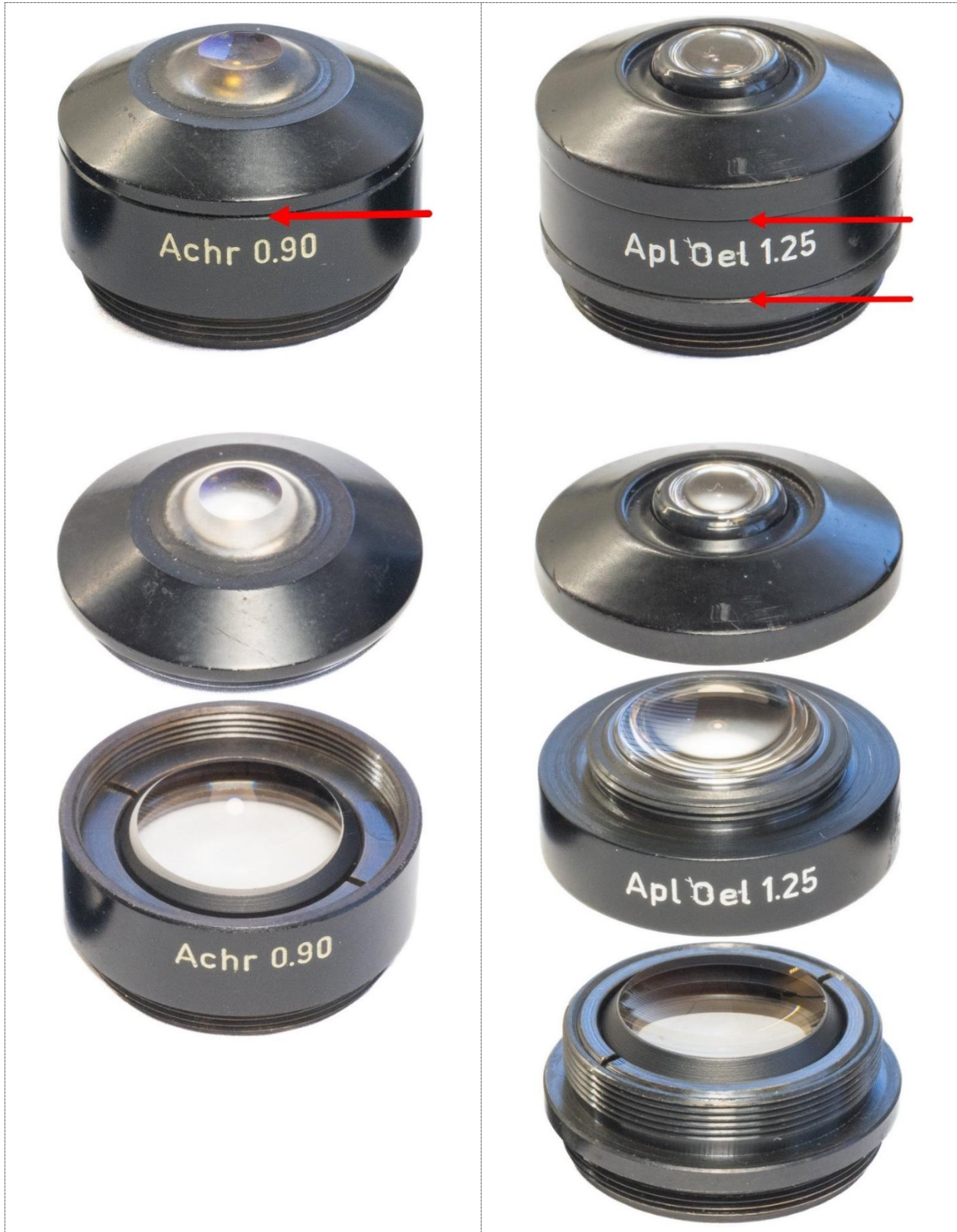
Figure 35: An aspherical-achromatic 0.90 n.a. top element (on the top of the image.) Below its two disassembled parts. The red arrow indicates the crevice between the top element parts.
