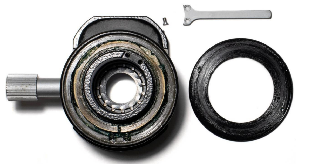
Figure 15: View of the condenser underside and the centering slide after the centering slide cover (on the right side) has been removed.
