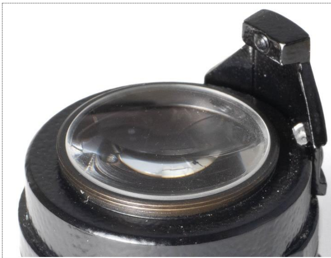
Figure 27: The top of the condenser core showing the primary condenser lens after the lens retainer has been removed.
