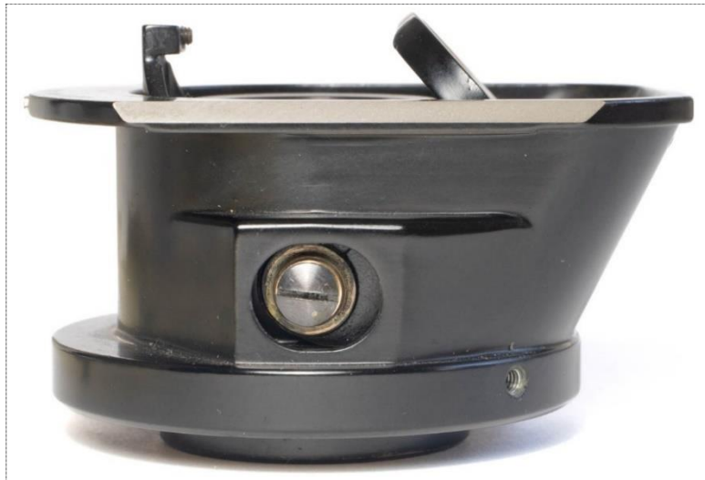
Figure 14: View of the side of the condenser casing (a.k.a. the "bathtub") after the swing-out knob has been removed.
