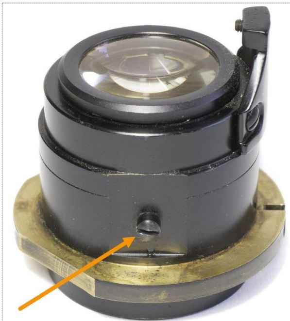
Figure 20: The removed condenser core viewed from the side. The arrow points to the pivot & guide screw that sits on the opposite side of the swing-out knob. (The top element yoke has prematurely been removed.)
