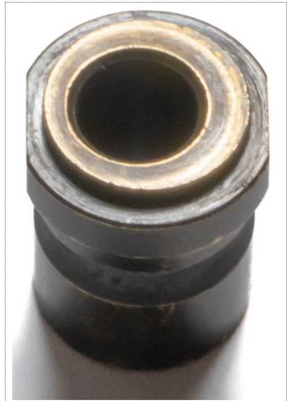
Figure 17: The condenser focus axle bearing. The image shows the excentricity of the axle hole and the parallel sides of the collar made to fit a thin wrench.
