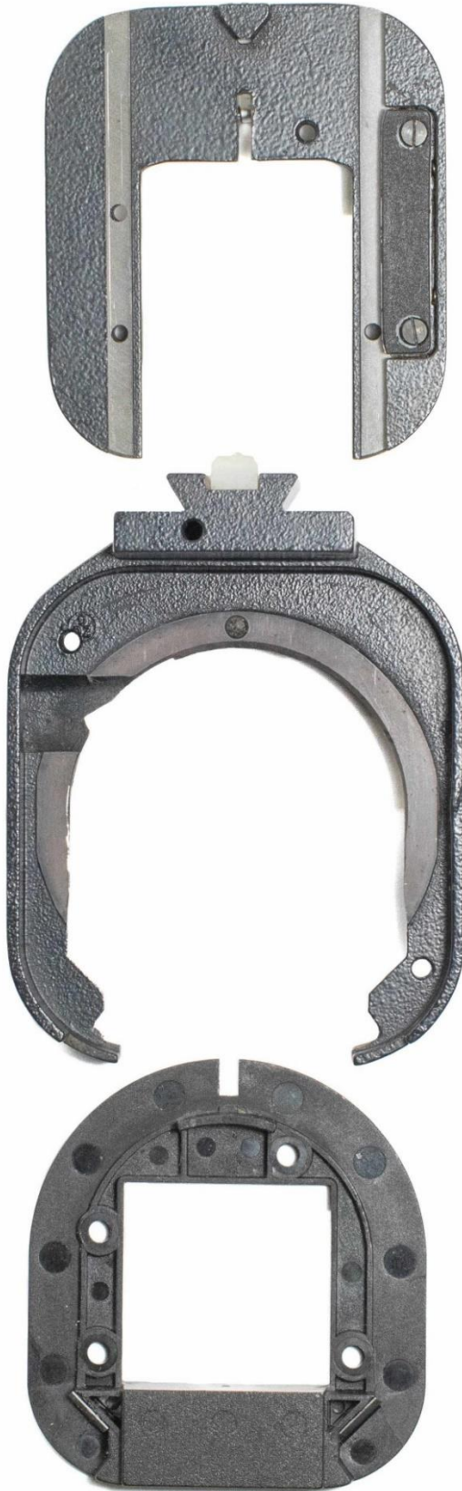
Figure 6: The main parts of the centering platform of the Laborlux family condenser holder viewed from the top.
