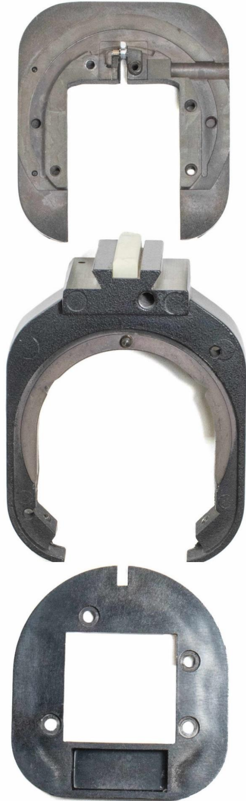
Figure 7: The main parts of the centering platform of the Laborlux family condenser holder viewed from the underside.
