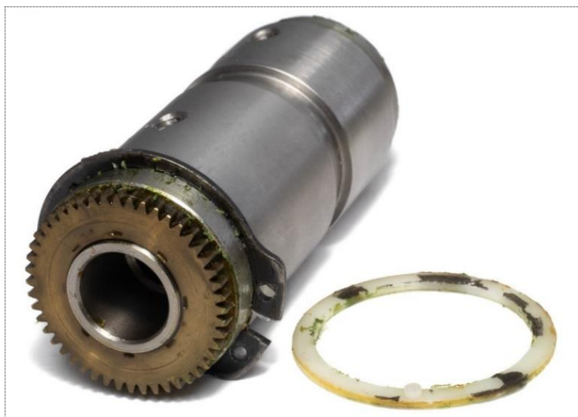
Figure 18: The left end of the focus cassette after it has been pulled off from the left coarse focus knob. The white plastic washer is attached to the snap ring.
