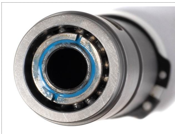
Figure 26: The right side of the focus cassette with the ball bearing assembled and freshly applied threadlocker (blue.)
