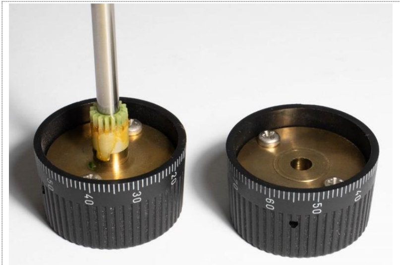
Figure 8: The fine focus knobs after removal. The fine focus axle remains attached to the left fine focus knob. Note the small screw hole on the side of the right fine focus knob.
