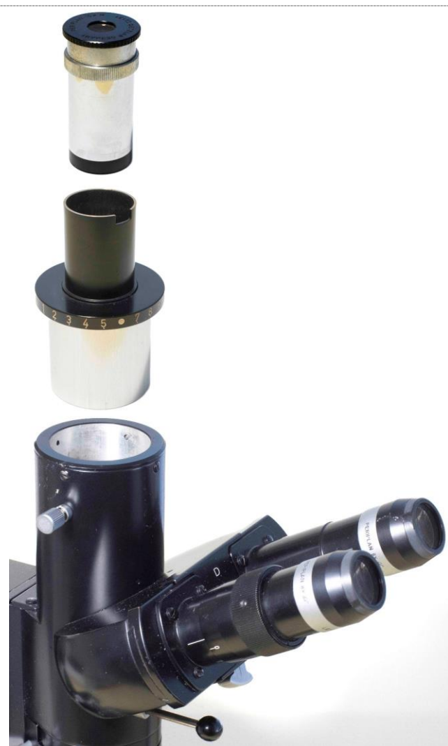
Figure 14: Trinocular microscope head with an exploded view of the phototube parts. From the bottom to the top: Trinocular head with 38 mm phototube, eyepiece adapter (38 mm → 23.2 mm), eyepiece.
