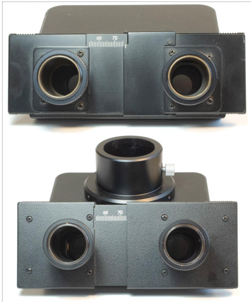
Figure 1: Two examples of different Leitz binocular/trinocular microscope head designs from the “160 mm tube length era”. (The eyepieces have been removed.)
