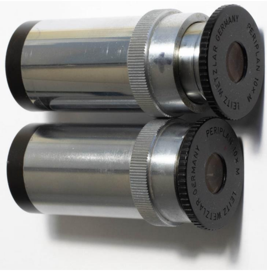
Figure 9: Focusable Leitz Periplan eyepieces with internal crosshairs. The image shows two identical eyepieces (of the older generation designed for a mechanical tube length of 170 mm) with different focus settings on the adjustable eye lenses.
