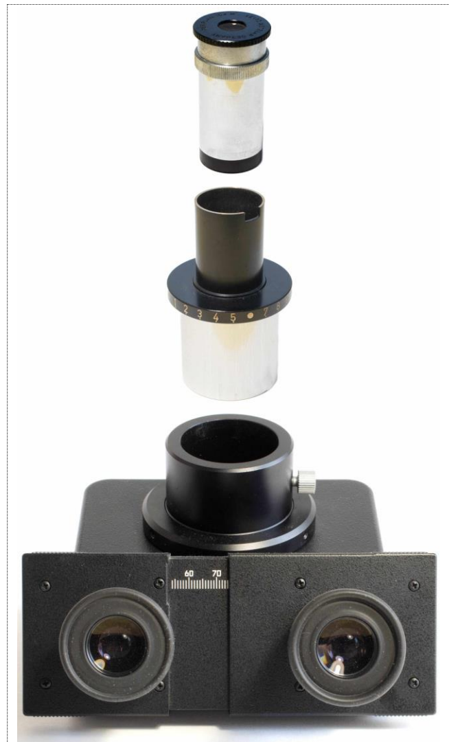
Figure 15: Trinocular microscope head with an exploded view of the phototube parts. From the bottom to the top: Trinocular head with a 38 mm phototube, eyepiece adapter (38 mm → 23.2 mm), focusable eyepiece with crosshair (the two last parts are of the older 170 mm tube length types.)
