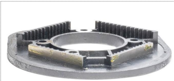
Figure 9: The bottom shell of the condenser holder viewed from the side of the buffer receivers. Note that the surfaces are covered with sheet metal plates that act as races for the buffer ball bearings.
