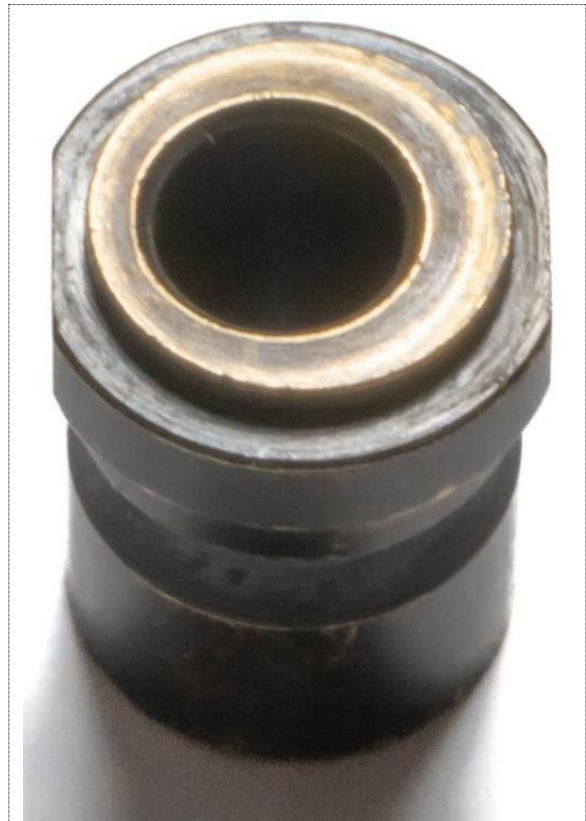
Figure 16: The condenser focus axle bearing. The image shows the eccentricity of the axle hole and the parallel sides of the collar made to fit a thin wrench.
