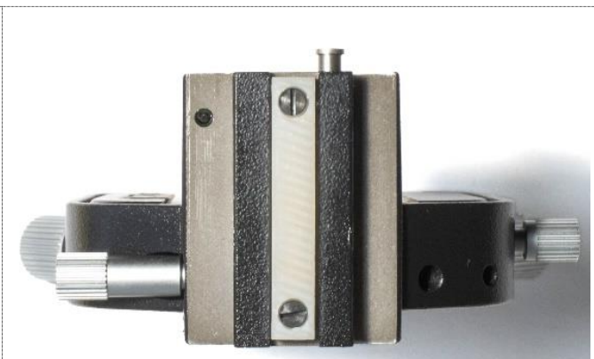
Figure 2: The backside of the condenser holder. The shiny knob to the left is for the adjustable condenser height stop. The top end of the stop rod is sticking up from the top of the holder. The condenser focus rack is the white, striped plastic part in the middle.
