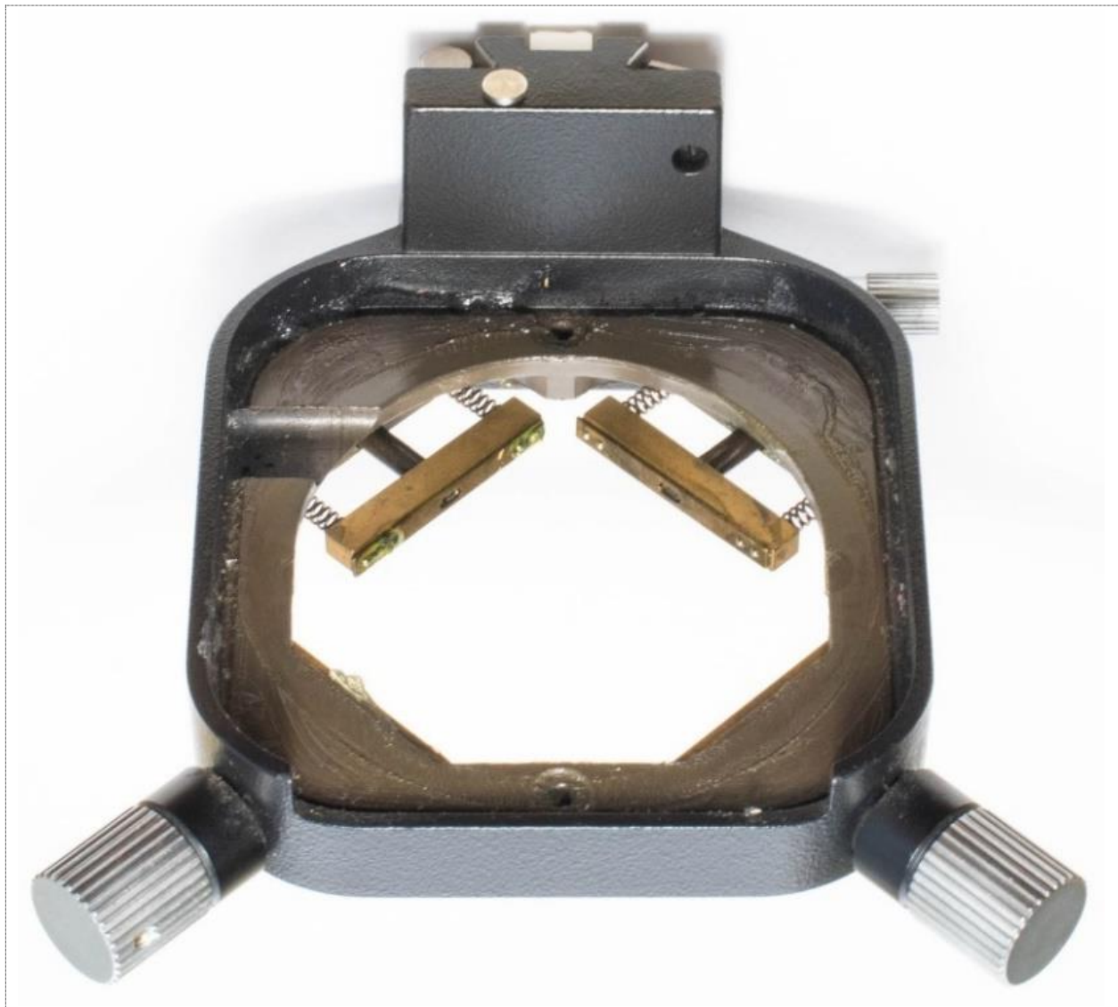
Figure 6: View of the condenser holder from the top and with both the bottom and the upper shells removed. Note the linear ball bearings on the front ends of the buffers. Each has four stainless steel balls that sit in a brass retainer.
