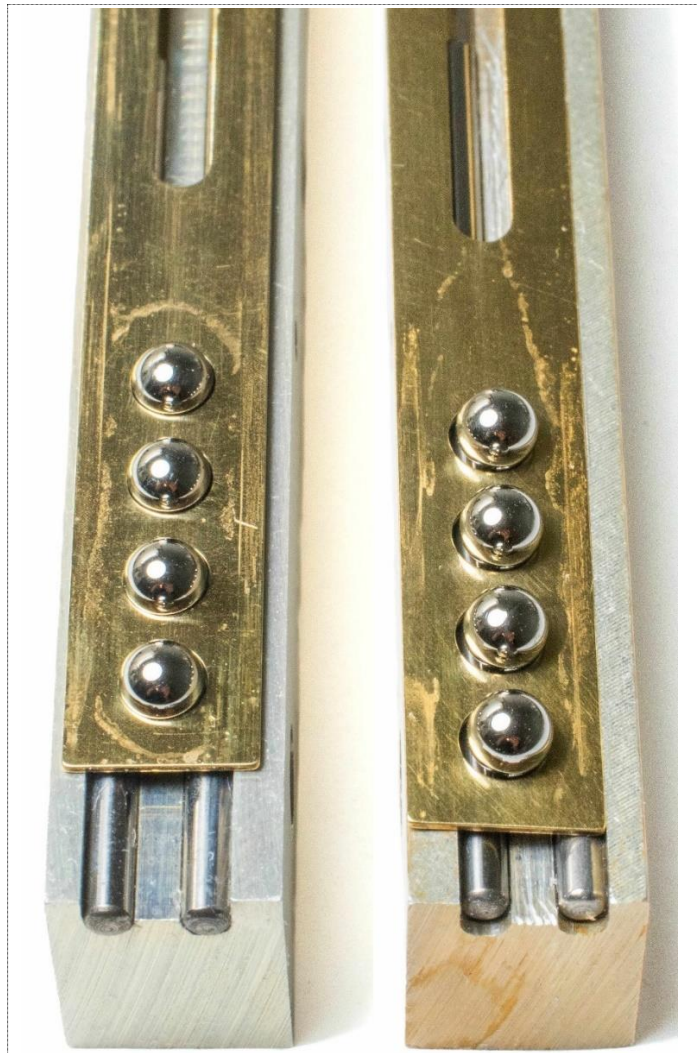
Figure 34: A properly seated bearing retainer on the left side and an erroneously seated retainer on the right side.
