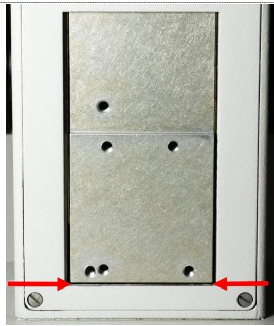
Figure 47: The focus slide set to its lowest position. The red arrows point to the 1 mm gap between the bottom of the focus slide and the lower edge of the focus slide cover.
