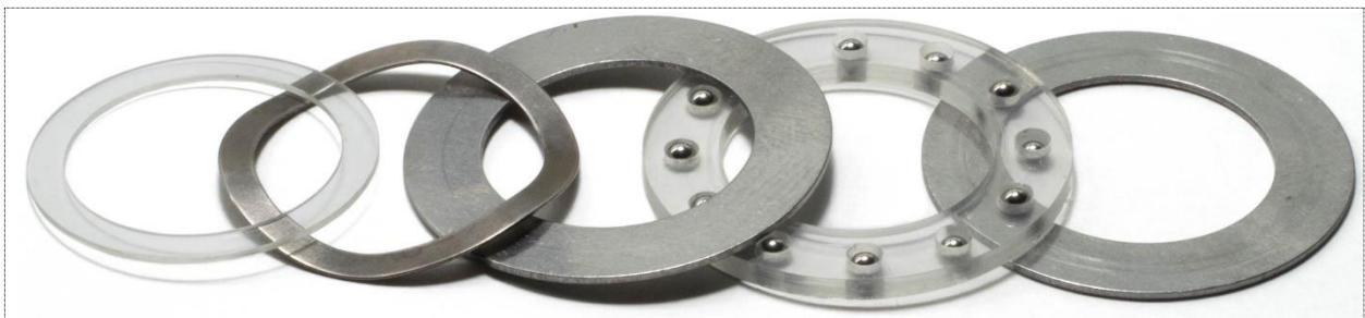
Figure 21: The two washers and the components of the axial ball bearing removed from the left end of the main focus axle.
