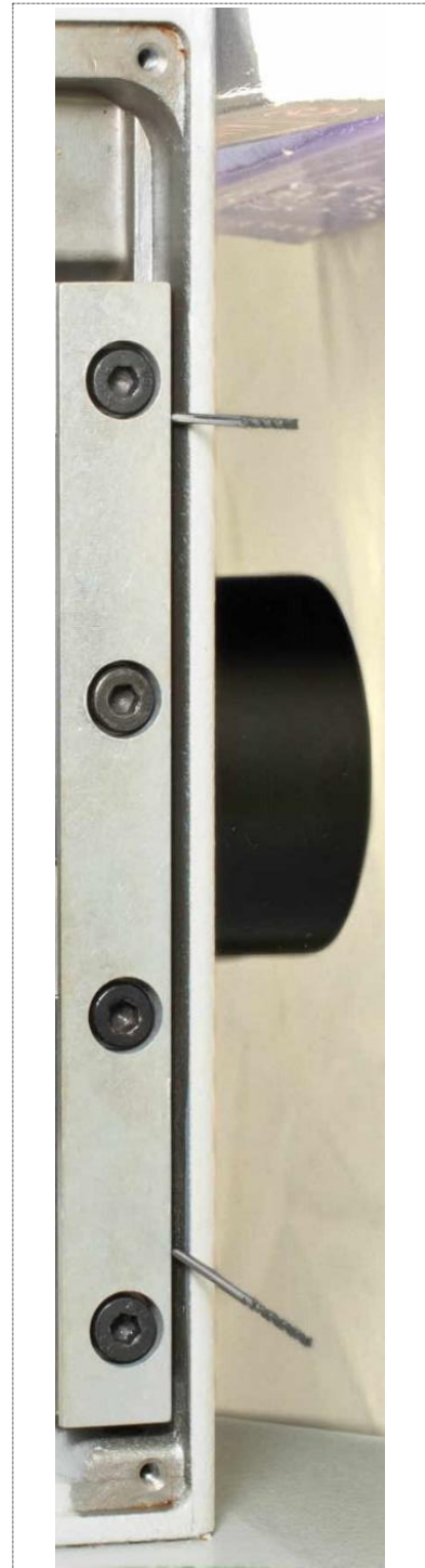
Figure 41: View showing how the temporary spacers (drill bits) are put between the inside of the focus slide bay and the right bearing guide.
