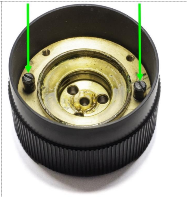
Figure 18: The inside of the removed left coarse focus knob. The green arrows point to the tall screw heads that are parts of the mechanism that limits the focus range.
