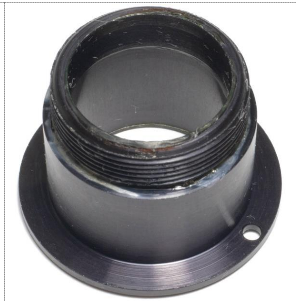
Figure 26: The black guide tube from the focus range limiting mechanism. The flange is facing downward in this image. The guide tube holds the stack of the 10 plastic rings (removed here.)
