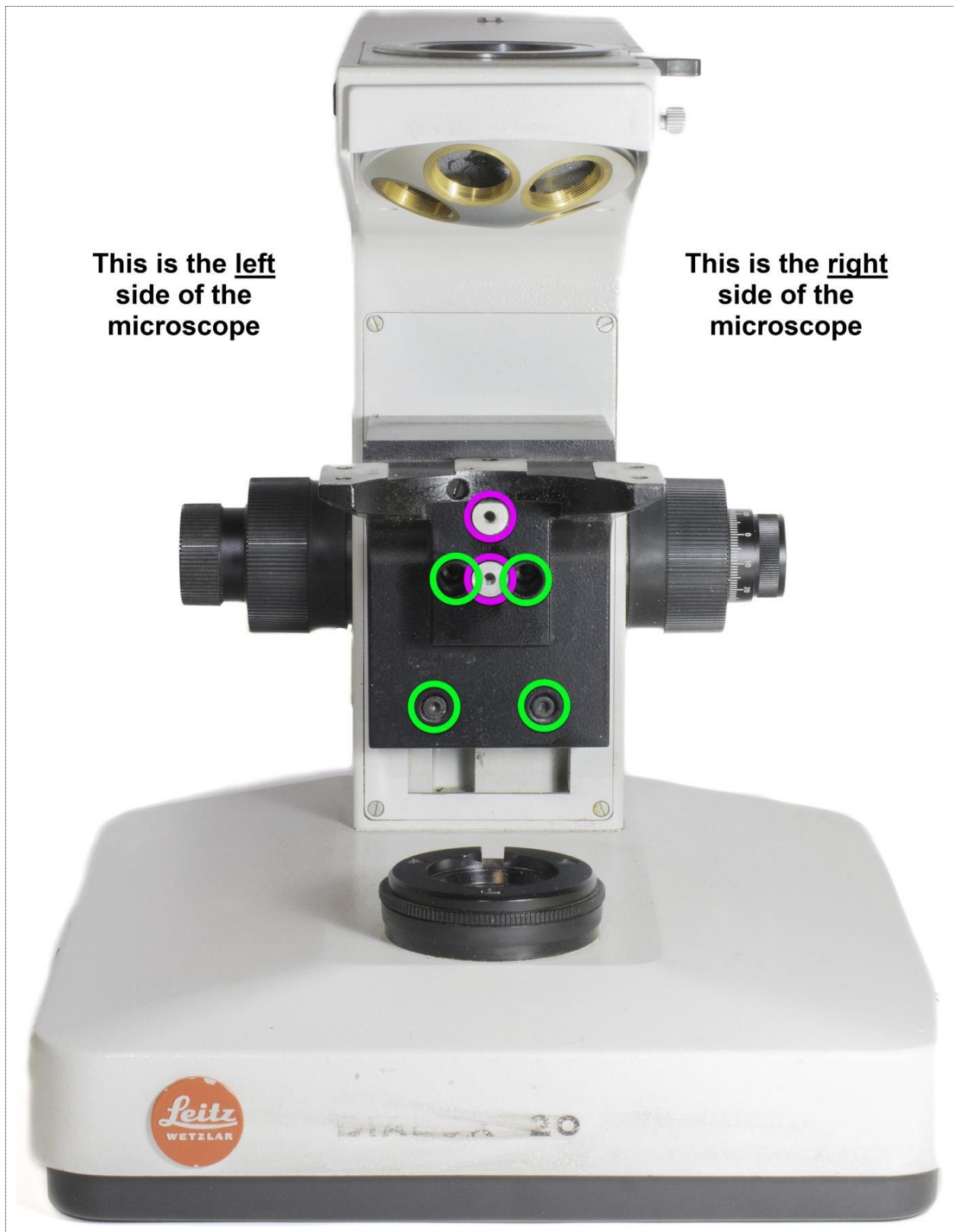
Figure 4: The microscope with the stage holder. The stage and the condenser assembly have been removed.
