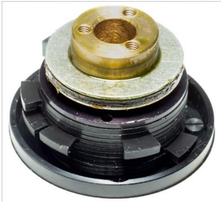
Figure 19: View of the left focus control base after the left coarse focus knob has been removed. The brass-colored part on the top is the left end of the main focus axle. Below is an axial ball bearing, a wave washer (not visible in this image), and then finally the 10 plastic rings that belong to the focus range limiting mechanism.
