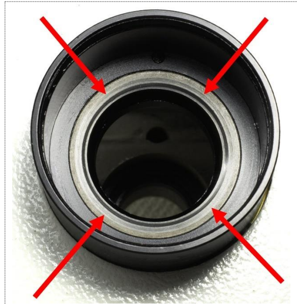
Figure 42: View of the inside of the right focus control base. The red arrows point to the stationary ball bearing race.
