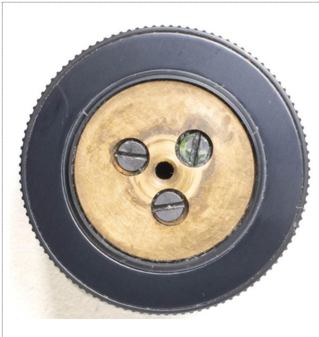
Figure 17: The face of the left coarse focus knob after the left fine focus knob has been removed. A bright imprint from the plastic washer that was between the knobs can be seen between the screw heads.
