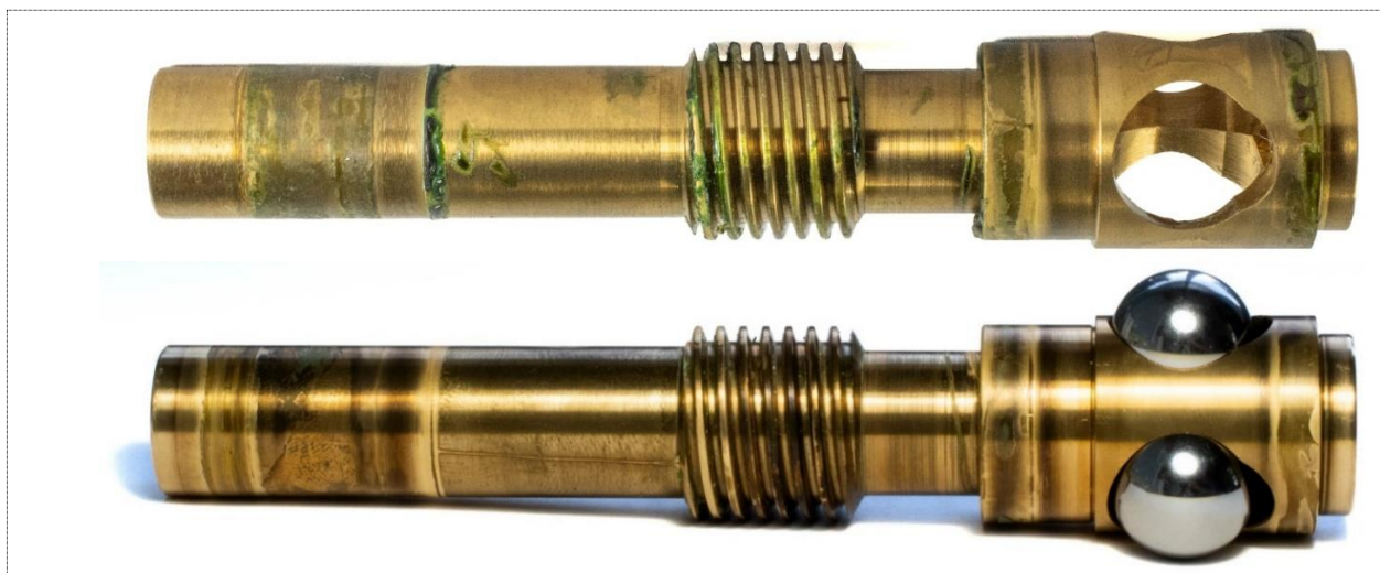
Figure 31: The main focus axle. The upper axle has green deposits of old hardened grease. The lower axle has the three large bearing balls still sitting in its right end. Both axles have tarnished patches from old grease.
