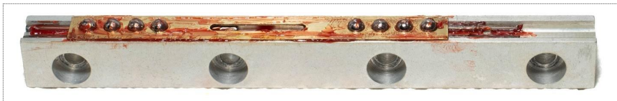
Figure 35: The focus slide's right bearing guide, greased, and with the bearing retainer and the bearing balls on top of the race. (The guide rests on two drill bits that are not visible in this image.)
