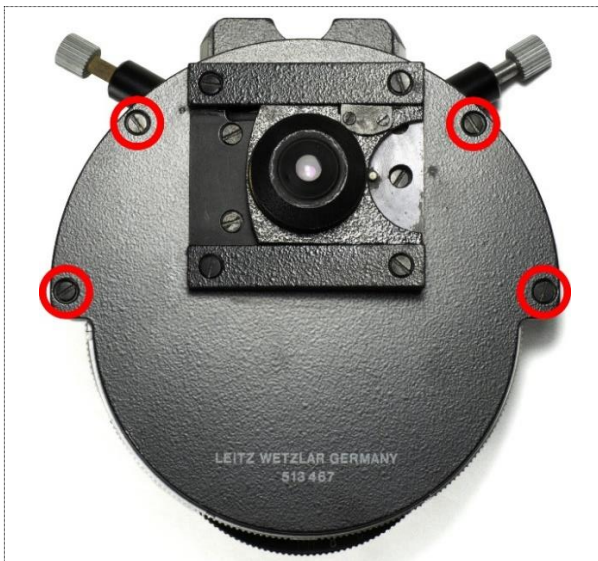
Figure 14: The UK condenser viewed from the top. The red circles indicate the screws that hold the condenser cover attached to the condenser casing.
