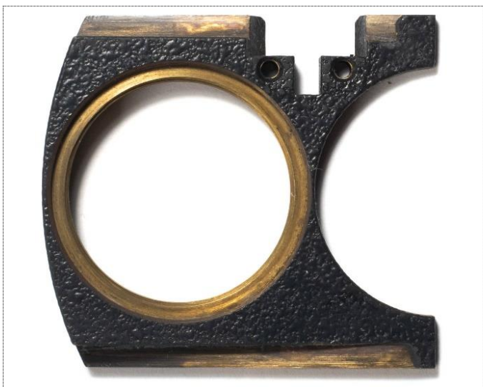
Figure 9: The top element holder. The catch has been removed from the holder.
