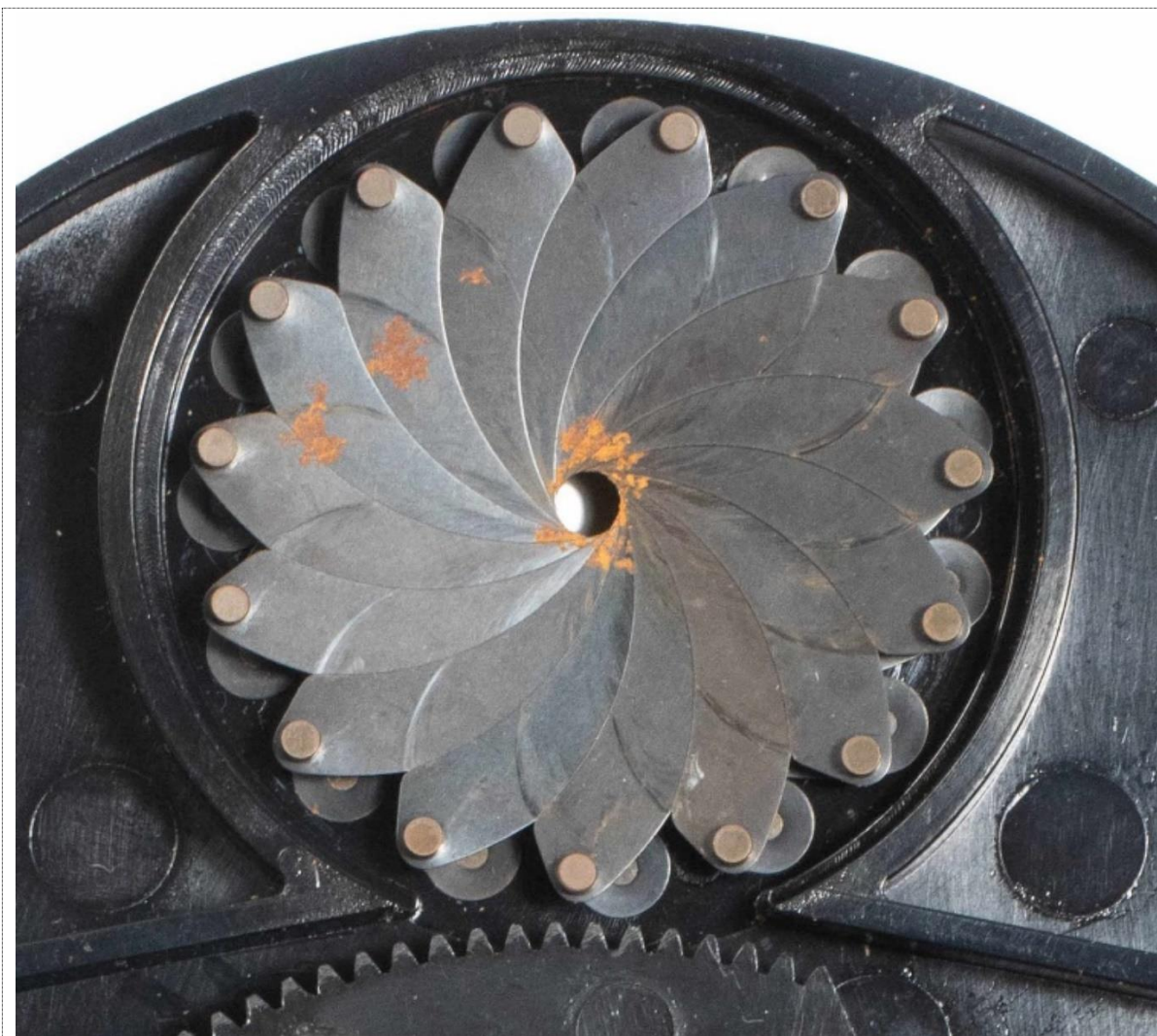
Figure 28: The aperture diaphragm blades after the actuator has been removed. The stationary sides of the blades are still sitting with their pivot pins in the holes in the turret base.
