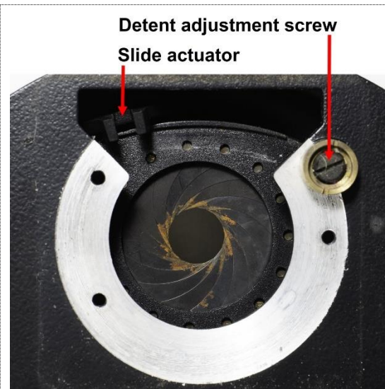
Figure 12: The top of the condenser cover after the top element base has been removed.
