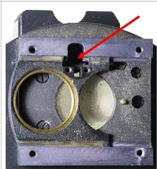
Figure 8: The top element holder on the top element base after the top element and both slide rails have been removed. The red arrow indicates where the top element catch must be positioned before the top element holder can be removed.
