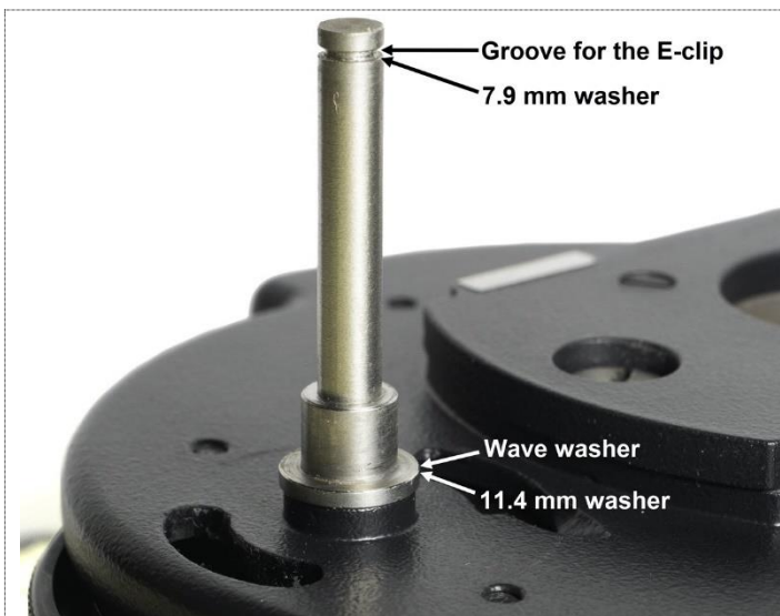
Figure 29: The grip axle on the underside of the condenser base. The arrows show where the E-clip and washers will be attached.
