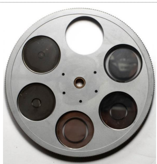
Figure 6: View of the underside of the light ring turret.
