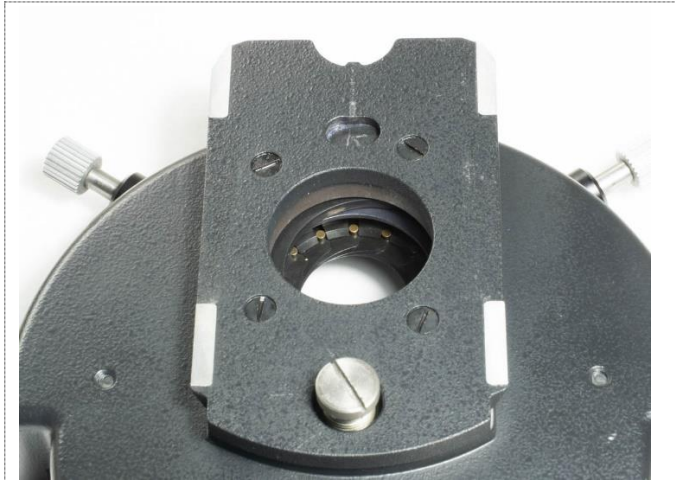
Figure 17: The underside of the UK condenser - looking at the aperture diaphragm below the dovetail sliding mount.
